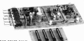
The 450 Tuner provides instant programme selection at the touch of a button ensuring accurate tuning of 4 pre-selected stations, any of which may be altered as often as you choose, by simply changing the settings of the pre-set controls.
