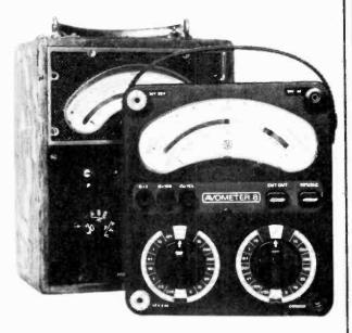
The Model 8 Mk 5 general purpose multi-range meter is the latest in a very long line of multimeters from AVO. An early version of the meter appears in the background.
