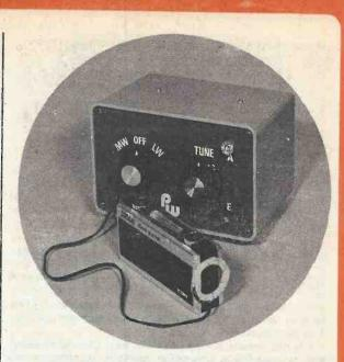
Here the output coil of the Signal Booster is placed close to the internal aerial of the transistor radio.
