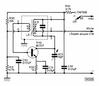
Fig. 11: Complete circuit of the BFO. The oscillator transistor Tr10 works at approximately 465kHz, frequency being varied by VC3, after rough adjustment of the core in L5.
