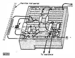
Fig. 115: Arrangement of Fig. 114 on T-Dec. Practical Wireless, September 1975
