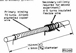
Fig. 113 : Construction of aerial coil on ferrite rod, used in experiments shown here.
