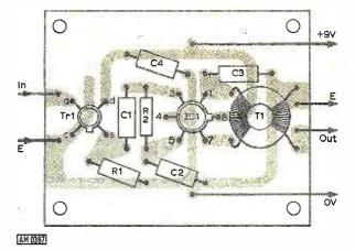
Fig. 5: PCB, full size, showing the component layout above and foil side below.
