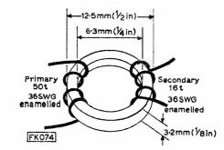
Fig. 4: Transformer T1, is of toroidal construction, efficient for broadband RF applications.
