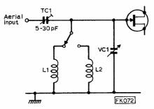
Fig. 1 : Alternative aerial coupling circuit to that used in the prototype, but of a simpler design.
