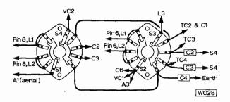
Fig. 10: Bandswitching for the Dual Conversion receiver is achieved with the wafer switch shown above. In the prototype only one wafer was used with contacts mounted both sides.
