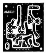
Fig. 2: Full size drawing of the printed circuit board viewed from the underside. Owing to its small size, considerable care should be taken in the drawing and etching of this board.
