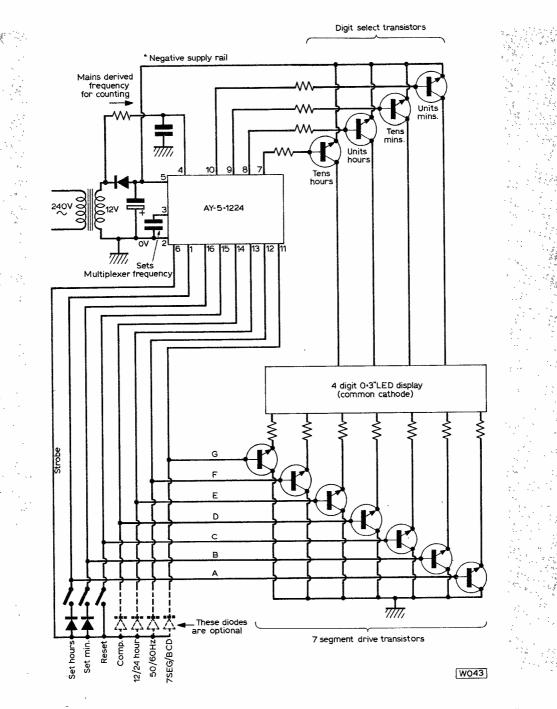
Fig. 1: General application circuit for the AY-5-1224 integrated circuit, emphasising the few components needed externally.
