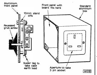
Fig. 3 : Suggested "safe" method of housing the Motor Speed Controller.
