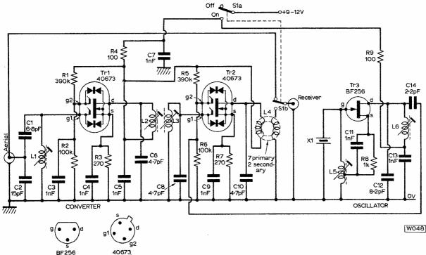
Fig. 1 : The complete circuit diagram of the converter. The oscillator circuit uses a crystal on 116MHz for easy calibration, while the output from the converter is via a wideband toroidal transformer.
