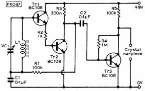
Fig. 118 ; above, shows addition of emitter follower stage to provide feedback.
