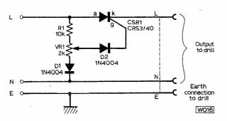
Fig. 1 : Circuit diagram of the Motor Speed Controller.
