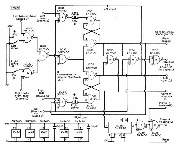
Fig. 1: Logic diagram of Board G which contains the new Serve/Lose logic. The (L) after some of the signals indicates negative logic (logic 1 = 0V). Fig. 2: below, Summary of connections to Board G from the original Tele Tennis Boards B and modified Board D (see Fig. 7).
