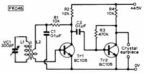
Fig. 116 : Circuit modification to retain high Q of tuned circuit.
