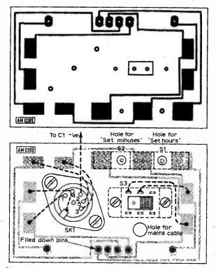
Fig. 3 left, and Fig. 4 above, show the end PCB's actual size and component layout. Fig. 4a below, shows the details of the two switches \$1 and \$2, constructed from phosphor bronze strip.
