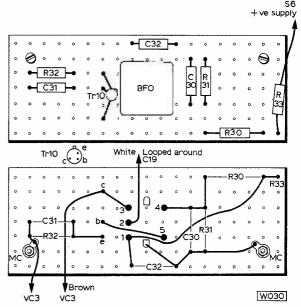
Fig. 12: Underside and topside of BFO board. The output signal is taken via an insulated lead, looped around C19.
