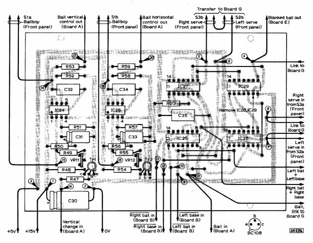
Fig. 7: Modifications to be made to the Board D in the original Tele Tennis unit.
