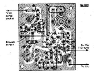
Component side view of the PCB, shown approximately  $1\frac{1}{2}$  times actual size. For components to fit the hole spacings correctly, the leads should be kept as short as possible.
