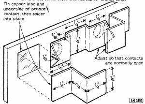
Insert and bolt into place SK1 and S3 then connect their tags to the copper lands of the board as shown in Fig. 4. With reference to Fig. 4a, cut and bend springy phosphor bronze (a piece of draught excluder strip will do nicely) into the shape of the contacts for S1 and S2. These contacts should be soldered on their respective copper lands having first tinned the underside of each contact where it comes into contact with the land. Now proceed to assemble the main board.
