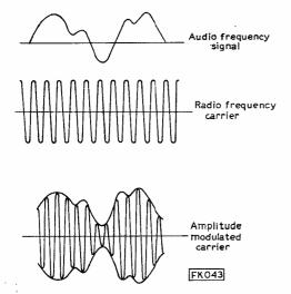
Fig. 112: Formation of an amplitude modulated (AM) signal from audio and RF sources.
