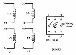
Fig. 2: L1/L2 coil winding details and pin configuration.
