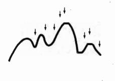
Fig. 2: Quantisation distortion. Wave-form of Fig. 1 distorted because number of bits (12) is insufficient to accurately represent amplitude levels as indicated by arrows in Fig. 1.
