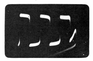
The same CRT displaying a 1kHz square wave. Astigmatism is most noticeable as is the lack of HF response due to the simple deflection amplifier.
