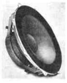
15" 14A/780. Bass unit on a rigid diecast chassis. Superior come material handles up to 50 watts RMS, and is treated to give a smooth frequency response. Resonance 30 Hz. flux density 360,000 Maxwells. Impedance at 1 kHz is 8 ohms. 3" voice coil.
