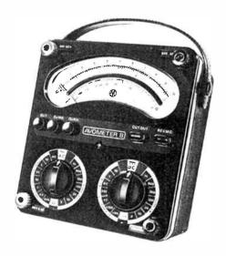
A large, clear scale with an anti-parallax mirror is the highlight of the latest AVO.
