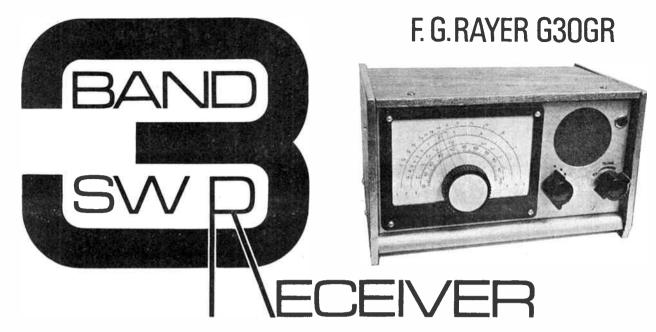
THIS receiver employs two transistors and two IC's, one of the latter in the intermediate frequency amplifier section and the second in the driver and output stages. It has band switching and covers all the important short wave ranges, including the low frequency bands, which are not included in some short wave or "all-wave" receivers.
