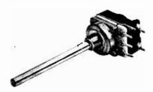
One of the Series C16 Cermet potentiometers by AB Electronic Components Ltd. Standard models range from  $100\Omega$  to  $2^\circ5M\Omega$ , linear, but special models down to  $50\Omega$  and up to  $10M\Omega$  are available, with soldering tags or printed circuit terminals.
