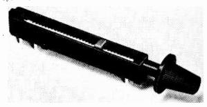
This 25-turn preset potentiometer by AB Electronic Components Ltd. is of carbon composition construction intended for use with varicap tuners. Resistance ranges up to  $100 k\Omega$  in linear, logarithmic or diode characteristic law.
