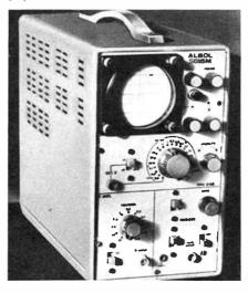
Bandwidth of the X amplifier, within 3dB, goes from d.c. to 3MHz, with an input impedance of  $1M\Omega$  in parallel with 45pF. The X deflection coefficient varies from 0·3 to 1·5V/cm. An attractive feature of this truly portable scope is that it can operate from 220 to 240V mains (using the optional adaptor) at 50 to 400Hz, with a power consumption of 40VA, or else from internal 1·5V cells giving 12V d.c. (rated then at 27W).
