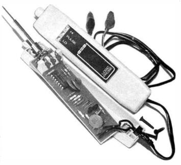
Construction proved to be very simple and straightforward, the step-by-step assembly instructions proving easy to follow. Unlike traditional British component placement drawings however this one did not show the copper track pattern of the p.c.b. and no holes are shown so that it is very important to check twice that the components are correctly placed.
