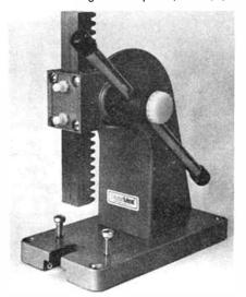
178mm high, is ideal for pressing bearings, forming and assembling small parts, staking rivetting and broaching. Built to stand the rigours of daily production line usage, the press has a rated capacity of 500psi.
