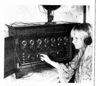
Apart from the usual aerial and anode tuning condensers the 2-V-4 included a special control for varying the bias voltage on the detector valve. Five plug-in coils were needed for each band covered so it can be imagined that a change of bands was not indulged in too frequently! A hefty 6V accumulator fed the valve filaments while the HT supply was around 60 to 100V.
