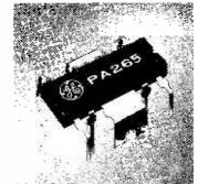
View of I.C. showing unusual heatsink tabs and staggered leads.
