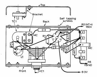
Fig. 2: Constructional details of the VFO assembly.
