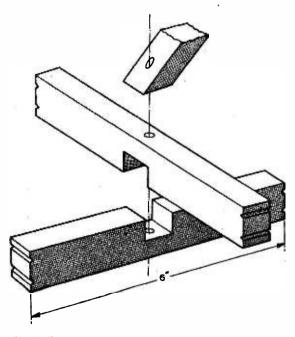
Fig. 1 : The construction of the search coil wooden framework.
