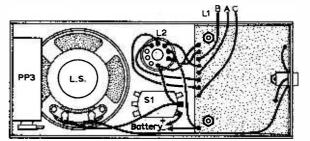
Fig. 6 : The wiring between the component board and the other components.
