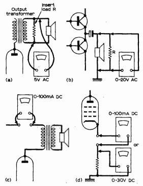
Fig. 2: Measuring output, (a) across dummy load or shunling speaker, (b) across speaker of transformerless stage, (c) current indication in series with anode load, (d) in series with cathode or voltage across blas resistor.
