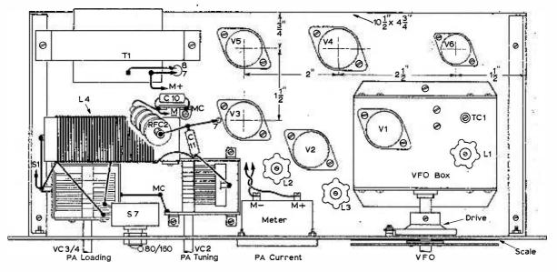
Fig. 3: Plan view of chassis showing disposition of major components.
