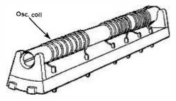
Appearance of typical coil biscuit. Oscillator coil is usually the largest and contains a tuning slug.
