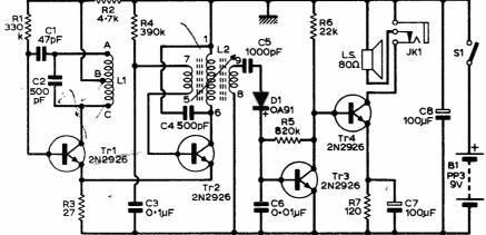
loudspeaker can lie between  $35\Omega$  and  $80\Omega$  and various miniature types with impedances in this range are available. If difficulty is experienced in obtaining one of these, the loudspeaker can be replaced by a transistor output transformer (such as the Eagle LT 700) feeding a lower impedance loudspeaker.
