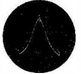
◀ Oscilloscope trace of response curve using wobbulator, with marker pip at top of curve (centre frequency f).
