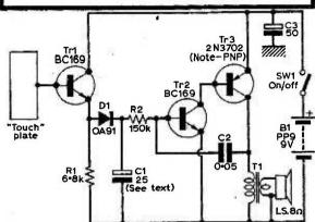
Fig. 1 : The circuit of the touch alarm
