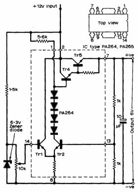
Fig. 1. Circuit of the PA264 with additional components required to provide 6v from 12v supply.
