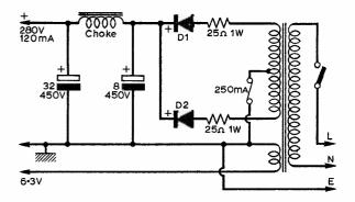
Fig. 6: Suggested power supply for the QRP transmitter.
