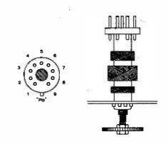
Fig. 3 : The pin numbering and mounting of L2.
