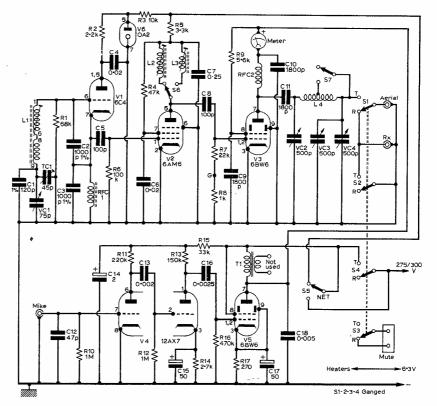
Fig. 1 : Complete circuit of the QRP transmitter.
