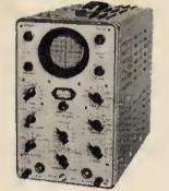
3-in tube fitted with telescopic viewing hood, giving bright display in full daylight. Bandwidth 10 c/s—10 mc/s. Triggered sweep pre-set at 1-2-5-10-30-100-300-1000-3000 µscc per stroke. Free-running time base 20 c/s to 2000ke/s with built-in crystal calibrator providing timing marks at .05-.2-1-5-20-100 µ scc  $\pm 5\%$ . Amptitude calibrator directly calibrated in volts. Input attenuator 1-10-100. Power supplies 127/230V AC.
