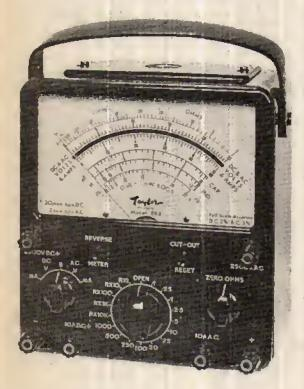
Fig. 3: The popular Taylor multimeter, Model 88B with a sensitivity of 20,000 ohms/volt d.c. and 2,000 ohms/volt a.c. Some idea of the scope range can be gleaned from the picture. Also see text.
