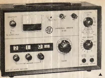
Fig. 13: For more advanced measurements and tests, this Universal Bridge by Avo, Model B.150, caters for a wide range of Inductance, capacitance and resistance measurements. Balanced null point is indicated by a meter, while the value of the component under test is automatically presented in digital form.
