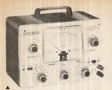
Fig. 7: Heathkit Audio Generator, Model AG-9U, Frequency range is from 10Hz to 100kHz with less than 0.1% distortion from 20Hz to 10kHz. Output voltage is indicated on a  $4\frac{1}{2}$ in. meter with three scales of 1 and 3 volts and --10 to +2dB.
