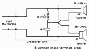
Fig. 1: The circuit of the cross-over network. The capacitor is a non-polarized electrolytic type.
