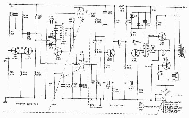
Fig. 3: Product detector, b.f.o., a.f. and output stages. The 5.6 volt stabilised line is taken to the junction of D1/R9 (Fig. 2).
