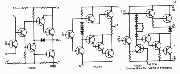
Fig. 1: Equivalent circuits of General Electric (U.S.A.) audio power integrated circuits.
