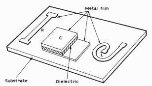
Fig. 2: Examples of a resistor, capacitor and inductor in thin film form.
