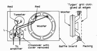
Fig. 3: Mounting and wiring of the speakers on the baffle board.
