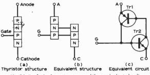
Fig. 21: Basic thyristor structure and the equivalent circuit.
