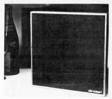
The 0.16 will handle loading up to 14 watts R.M.S. and presents an 8 ohm impedance to the amplifier output. Frequency response extends from 60 to 16,000Hz with exceptional smoothness. A specially designed driver system is used in a sealed and contoured pressure chamber to ensure good transient response at all frequencies. Size: 9<sup>2</sup>/<sub>3</sub> square × 4<sup>3</sup>/<sub>3</sub> deep from front to back.
