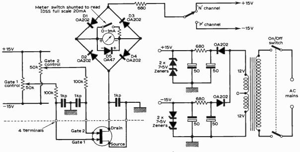
Fig. 4: Circuit of the f.e.t. tester.
