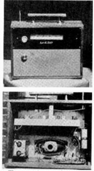
The two photographs are of a v.h.f. portable comprising the PRACTICAL WIRELESS V.H.F. Tuner (Feb.-March 1968) and basic amplifier (November 1967).
