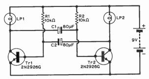
Fig. 1 : The circuit of the light flasher.
