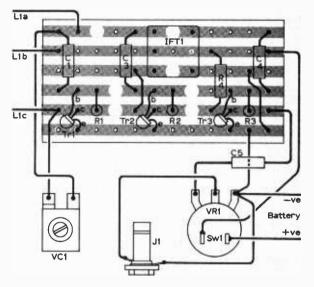
Fig. 2: The component layout inside the soap box.
