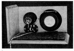
The partially assembled enclosure.
