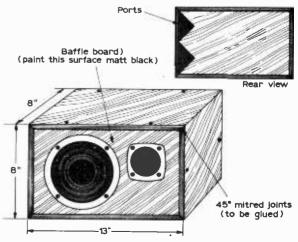
Fig. 2: The assembled enclosure.
