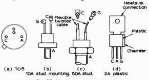
Fig. 23: Thyristor encapsulations.
