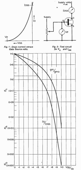
Fig. 3 : Normalised curves for  $I_{\rm D}$  and  $g_{\rm M}$  versus  $V_{\rm GS}$
