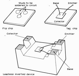
Fig. 3: Three types of device construction for use with thin film circuits.
