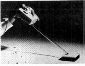
The prototype of the metal locator.
