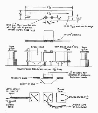
Fig. 1: The constructional details for fitting an extra tape head.
