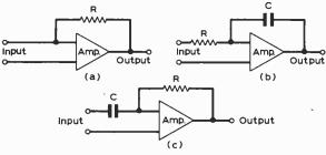
Fig. 1: Operational amplifier applications
