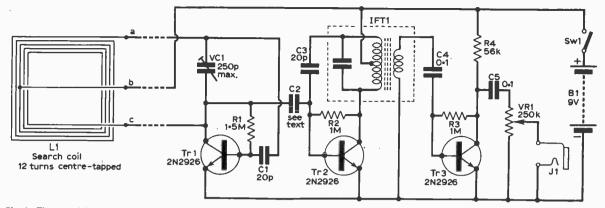
Fig. 1: The complete circuit of the metal locator. Note that C2 is not a physical component as it is stray capacitance; it is drawn here to simplify the explanation.
