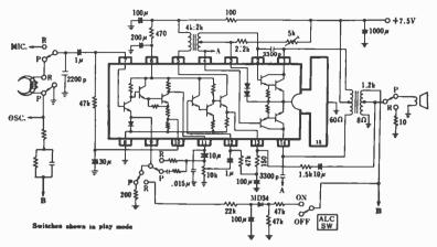
pre-amp and driver sections. The circuit consumes only 15mA under zero signal conditions. The whole device is packaged in plastic dual-in-line and will operate over the temperature range  $-10^{\circ}$  to  $+125^{\circ}\text{C}$ .
