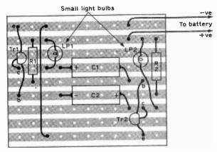
Fig. 2: The component layout on a small piece of Veroboard.
