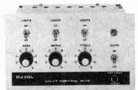
3 channel light control unit that handles up to 1,000 watts per channel. Separate bass, middle and treble controls for full frequency senaration
