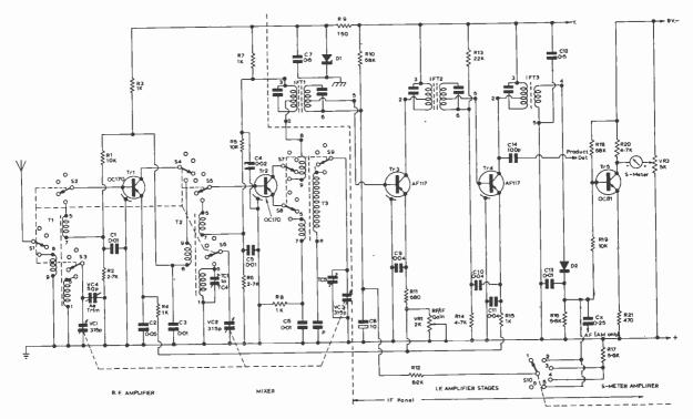
Fig. 2: R.F., mixer, i.f. and meter amplifier stages. See text p.870 for values of padder condenser P. Note: S6 should be shown as ganged to S8.
