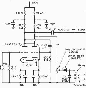
Fig. 1: The circuit of the Vox Control Unit.
