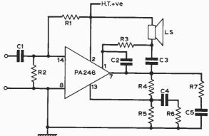
Fig. 2: Practical circuit for the PA246 with 5 watts audio output. Alternatively, the PA237 may be used but the audio output will be 2 watts. Capacitor C3 is an electrolytic—the plus side should be taken to the junction of R3 and the loudspeaker.
