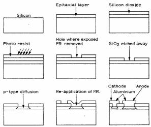
Fig. 1 : Planar technology : the stages involved in the manufacture of an epitaxial planar diode.
