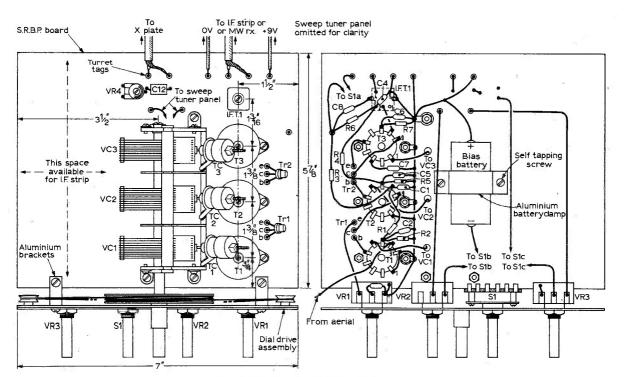
Fig. 6: The layout and wiring diagram.
