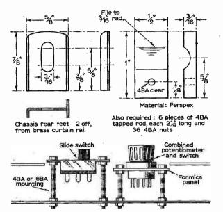
Fig. 4: Details of the sub panels, control mountings, chassis feet and I.w. trimmer capacitor support. Tag panel A is shown on the left, panel B on the right.
