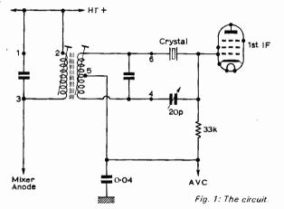
The crystal was 464.75kHz, obtained from the supplier listed. There is no need to use this exact frequency, as all the i.f.t.s are later aligned on the crystal frequency.
