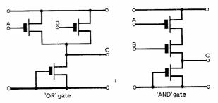
Fig. 5: MOST logic gates.
