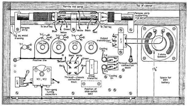
Fig. 5: (above) The component layout viewed from the rear of the case, the drilling plan is shown in Fig. 2.
