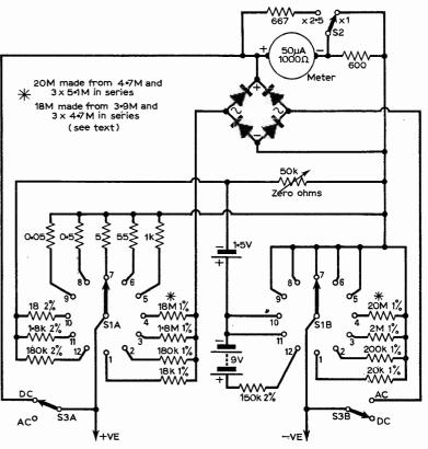
Fig. 1: The complete circuit of the Microtest.
