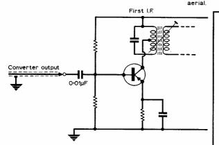
(d) Converter coupled to a 1-6MHz I.F. strip. Fig. 9: Coupling arrangements for the Panadaptor—see text for explanations.
