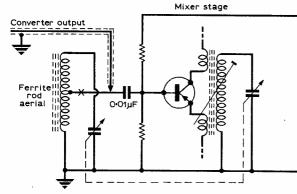
(b) Alternative method of coupling to by pass the ferrite rod
