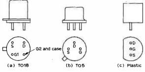
Fig. 18: F.E.T. encapsulations.
