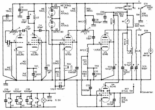
Fig. 1: The complete circuit of the transmitter.
