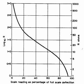
Fig. 2: Resistance measurements can be calculated from a graph stuck on the bottom of the case.
