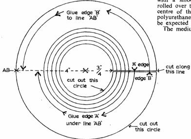
Fig. 6: Diagram showing how a sheet of card should be cut and glued to form a small h.f. radiator for the centre of the large cone.
