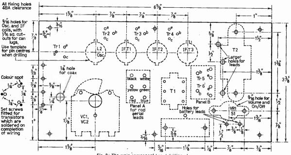
Fig. 2: The main component board drilling plan.
