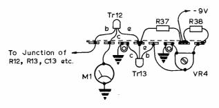
Fig. 47: Component layout and wiring for the 'S' meter circuitry.
