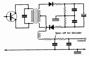
Fig. 11: Typical discriminator output (transistorised tuners).
