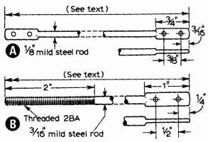
Fig. 19: Coupling rods. (A), to lever rollers. (B), to pedals.
