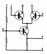
Fig. 1: The integrated circuit under review this month is the CA3028 manufactured by R.C.A. The theoretical circuit, containing three transistor elements, is shown alongside.
