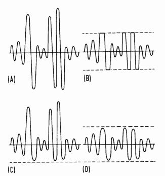
(A) A typical incoming audio signal with noise peaks apparent.
