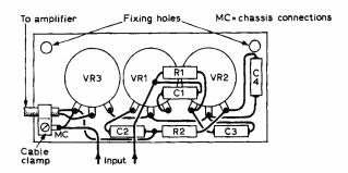
Fig. 2: The wiring of the tone control panel.
