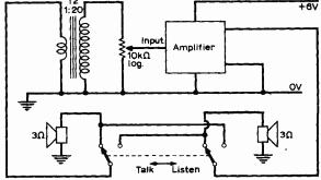
Fig. 6: Schematic of the amplifier used as an intercom.
