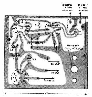
Fig. 3: The printed-circuit layout for Fig. 2, seen from the copper side.
