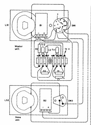
Fig. 2: Component layout and wiring details
