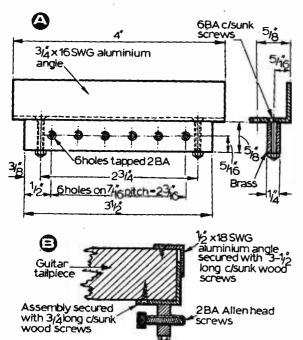
Fig. 13: Details of the forward stop bar fitted beneath the tail end of the guitar body.
