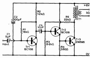
Fig. 1: The circuit of the transistor amplifier
