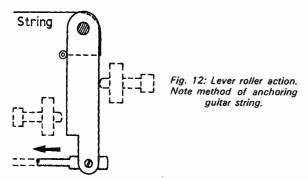
between the bridge and the tailpiece? This has been tried and rejected for the simple reason that strings continually tensioned and de-tensioned across the edge of a bridge very quickly break. The method described in these articles is basically the same as that developed for commercially-made instruments now on the market and overcomes this problem.
