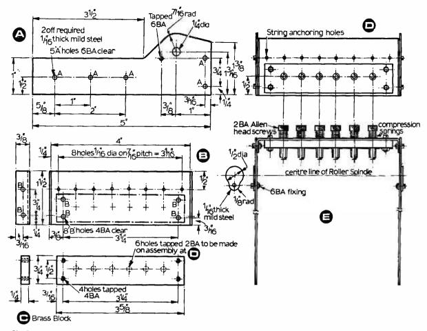
Fig. 9 (above): (A) Side of frame—two required. (B), (C) Tail plate assembly. (D) Holes for the 2BA Allen screws drilled and tapped after brass block is fitted as in (C). (E) Final assembly of the roller bridge frame. Note retaining caps for roller spindle.
