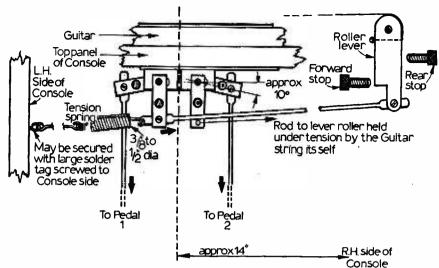
Fig. 15 (above): The action of the lever roller and pedal coupling mechanism situated beneath the top of the consol. Arrows show movement of rods when pedal 1 is pressed. Text explains mechanism.
