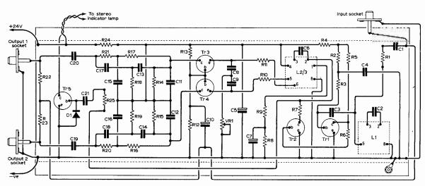
Fig. 5: Wiring and layout of decoder (Mullard Coils).
