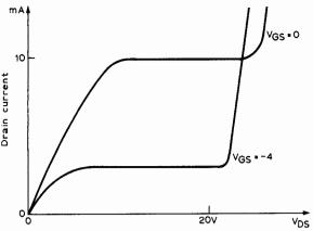
Fig. 3: Curves showing variation in drain current with drain voltage for different gate voltages.
