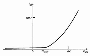
Fig. 5: Enhancement-mode insulated gate field effect transistor characteristic curve.
