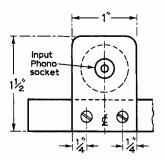
Fig. 3a: (above left) Output socket assembly. Fig. 3b: (above) Input socket assembly.
