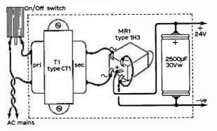
Fig. 9: Power supply assembly details.
