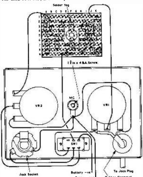
Fig. 2: The rear view chassis layout and component grouping on the Veroboard. The soldering tag connects to F1.
