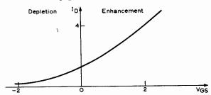
Fig. 7: Curve of drain current against gate voltage for a depletion mode i.g.f.e.t.
