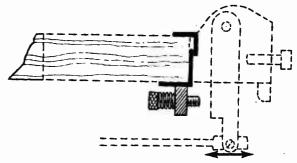
Fig. 14: Position of forward stop bar relative to the bridge frame and lever rollers.
