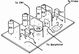
Fig. 4: The circuit panel, showing where components are mounted.
