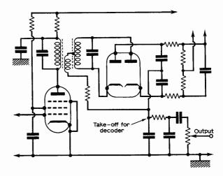
Fig. 10: Typical discriminator output (valved tuners).
