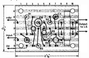
Fig. 2: The component layout on the Veroboard.
