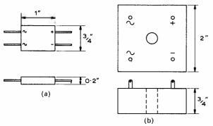
Fig. 11: (a) 1.8A and (b) 10A bridge encapsulations.
