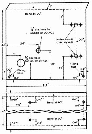
Fig. 4: A small chassis and panel suitable for the i.c. tuner.
