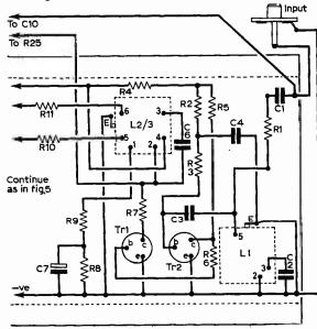
Fig. 7: Coil wiring for Henry's Radio decoder coils.
