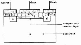
Fig. 6: Depletion-mode i.g.f.e.t. construction.
