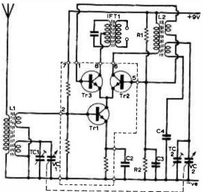
Fig. 2: The CA3028 can be used as a combined r.f. amplifier, mixer and oscillator in a receiver front-end. This particular circuit is for a short-wave tuner to go ahead of a medium-wave receiver.
