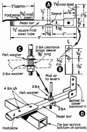
Fig. 18: Dimensions and assembly of foot pedals.
