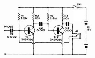
Fig. 1: The Injectrace signal injector and tracer. Functions are changed merely by plugging in the earphone.
