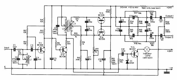
Fig. 1: Circuit diagram of the stereo decoder.
