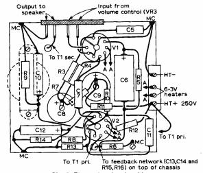
Fig. 3: The under chassis wiring.
