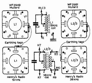
Fig. 6: Outlines and connections of available coils.
