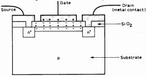
Fig. 4: Structure of an enhancement-mode insulated gate field effect transistor.
