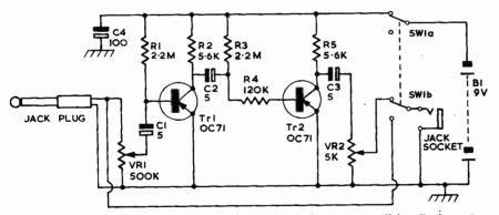
Fig. 1: The audio noise limiter using transistors biased almost to cut-off for clipping noise.
