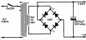
Fig. 8: Circuit of the power supply.
