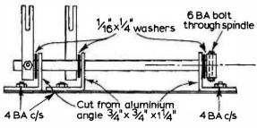
Fig. 17: Side view of mechanism shown in Fig. 9A.
