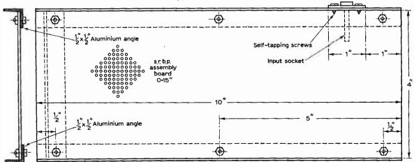
Fig. 2: Assembly board and support rails.
