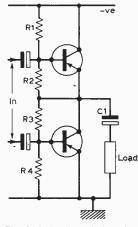
Fig. 6: A single-ended pushpull or totem-pole amplifier.
