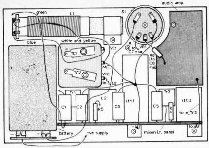
Fig. 2: General layout and inter-module wiring.
