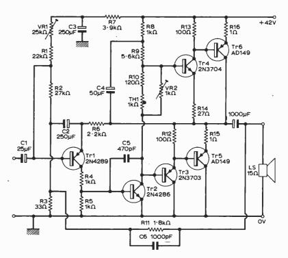
Fig. 1: The circuit of the power amplifier.
