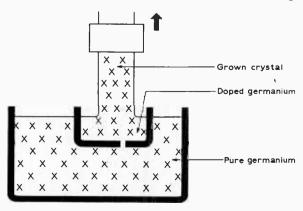
Fig. 5: The double-crucible method of growing doped crystals.
