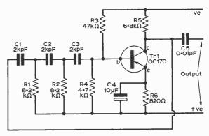
Fig. 1: The circuit of the phase shift oscillator. The voltage is 9v, supplied by any battery.
