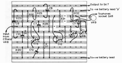
Fig. 8: Layout of the amplifier panel.
