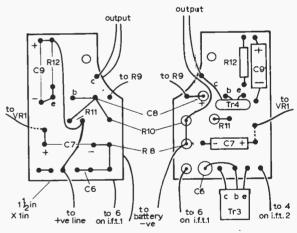
Fig. 4: The detector and audio stages.
