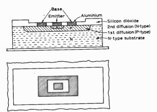
Fig. 5: Epitaxial planar transistor construction.
