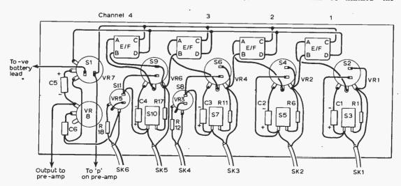
Fig. 7: Wiring of the main panel.
