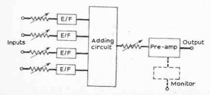
Fig. 1: Block diagram of an active mixer.
