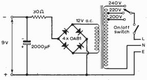
Fig. 9: A suitable power supply.
