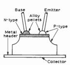
Fig. 1: Mesa transistor construction.
