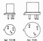
Fig. 2: Typical low-power transistor encapsulations.
