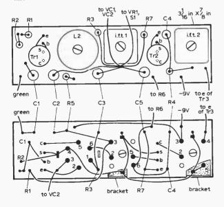
Fig. 3: The r.f. and i.f. amplifier component board.
