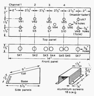
Fig. 5: Dimensions of cabinet, side panels and screens.
