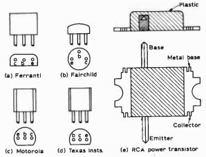
Fig. 6: Common epoxy resin encapsulations.
