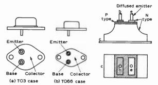
Fig. 3: Power transistor encapsulations.
