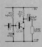
Fig. 1: A single-ended stage using thermistor compensation. If the voltage at A is less than half the line voltage, thermal runaway cannot cause damage. R3 may be used as the load if bias current can be passed through the load (not suitable for use with a loudspeaker)
