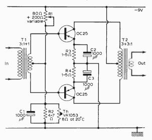
Fig. 4: A push-pull transformer coupled amplifier.
