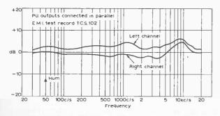
Fig. 2: The equilisation of the unit for a Deram pickup.
