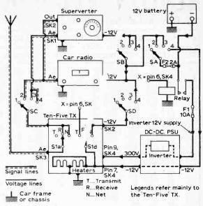
Note: A panel-fitted on/off switch is also required between tag T'S1d and pin7, SK4 to produce HT for Netting when necessary.
