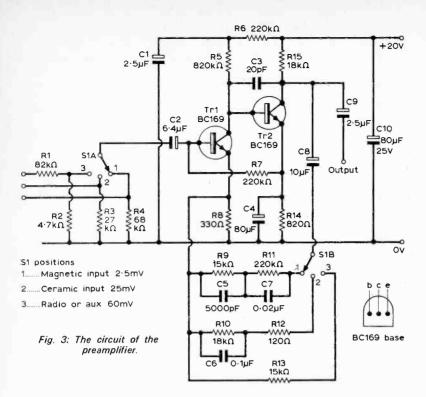
For ceramic cartridges the low and high turnover points can be adjusted by altering the input resistor R3. The value shown gives a good response for the Sonotone 9TAHC, while the graph shows the curve for a Deram pickup.
