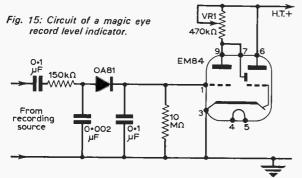
provide some method of indicating the strength of the applied signal. This is frequently done by means of a "magic eye" valve and for constructors who wish to employ this method, the circuit is given in Fig. 15. The reference signal is taken via a 0·1mfd condenser from the same point as the record signal
