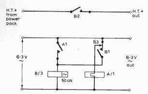
Fig. 4: A method of automatically delaying switch-on of an h.t. line. Notice that the thermal relay A/1 is taken out of circuit when B/2 operates, so that it can cool for the next time it is used.
