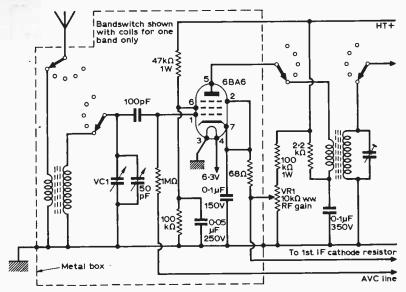
Fig. 6: The circuit of the r.f. stage.
