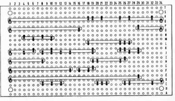
Fig. 4: The component layout of the preamplifier showing the positioning of the Cir-Kit strip.
