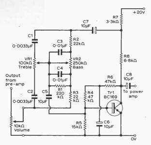
Fig. 5: The circuit of the tone control.
