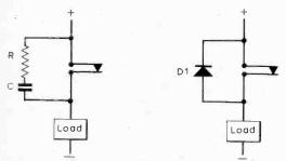
Fig. 1: Spark suppression of relay contacts for inductive loads.
