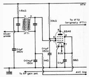
Fig. 7: The circuit of the additional i.f. stage.
