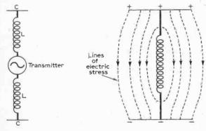
Fig. 1: The electric field with no aerial current.
