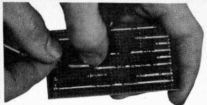
Laying the Cir-Kit strip is a simple matter of peeling back the protective backing and pressing it onto the matrix board.
