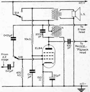
Fig. 14: The output pentode may be used in the circuit shown for providing erase and bias current while recording.
