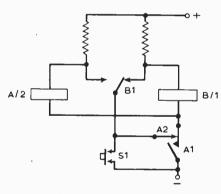
Fig. 5: A relay scale-of-two circuit.
