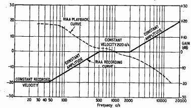
Fig. 5: RIAA recording---playback curve.
