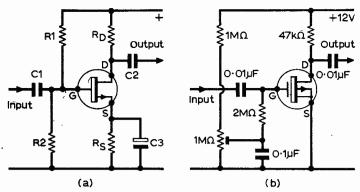
Fig. 3: (a) The biasing of a n-channel JGFET of the enhancement type; (b) alternative method of biasing an IGFET of the n-channel type.
