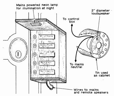
Fig. 9: Constructional details of the multispeaker buzzer system.
