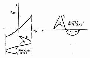
Fig. 8: Transfer characteristic of a typical amplifier, showing effect of intermodulation distortion.
