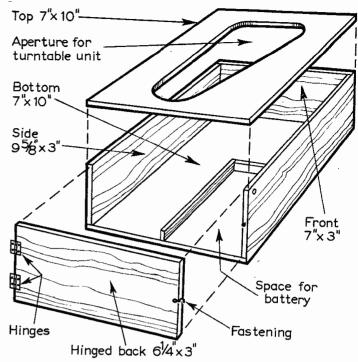
Fig. 4 (above): Case construction details Fig. 5 (below): Motor and pickup connections
