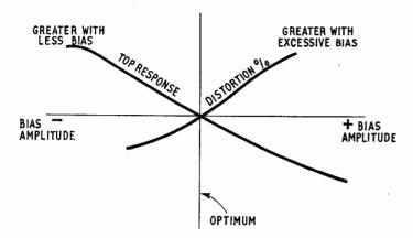
Fig. 9: Bias setting is important for tape recorder adjustment.
