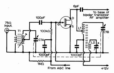
Fig. 4: JGFET arranged as a v.h.f. amplifier, tunable over Band II. The a.g.c. input is at the gate, via the 100k $\Omega$  and 1M $\Omega$  potential divider.
