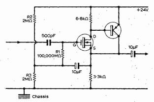
Fig. 6: Hybrid f.e.t./bipolar circuit with ultra high input impedance.
