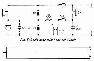
Fig. 7: Shorthand way of showing the circuit of Fig. 6.
