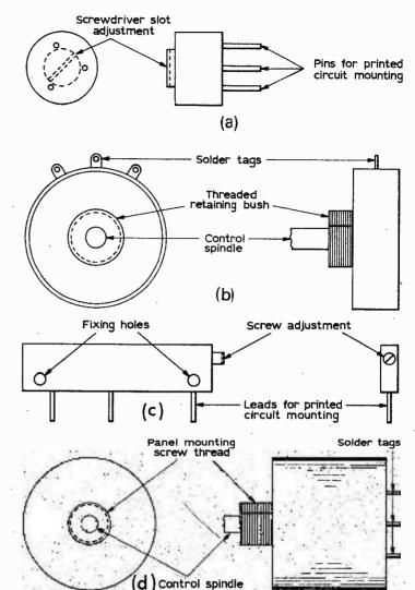
Fig. 5: (a) Printed circuit mounting potentiometer, (b) panel mounting potentiometer, (c) flat printed circuit multiturn potentiometer, (d) precision helical multiturn potentiometer.
