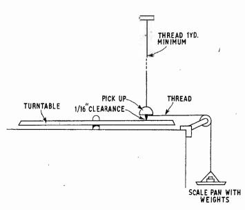
Fig. 2: Method of measuring back bearing friction.
