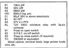
constructional details is shown in Fig. 12. The timer is designed to do the following: (1) Switch on the enlarger for three separately set times (successive exposures through red, green and blue filters). (2) Give an audible signal at the end of three different preset periods of 3, 1 and 2 minutes (developer, stop and bleach-fix bath times).
