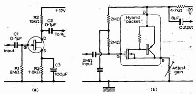
Fig. 2: (a) Simple a.f. amplifier using a JGFET of the depletion type; (b) hybrid "packet" in which a p-channel IGFET is integrated with a n-p-n bipolar transistor, giving a 2MΩ input impedance and medium output impedance with very high signal gain.
