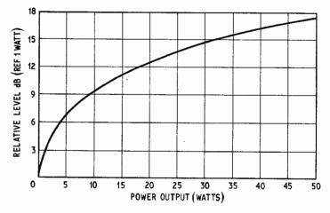
Fig. 11: Loudspeaker efficiency. Graph showing relationship between power input and sound pressure, reference 1 watt.
