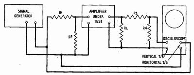
up the gain to distortion point, then back off slightly and note the output meter reading. Feed a 1kc/s signal to the pickup input and set the generator input for an output reading 20dB or so below the previous reading and take this as the OdB level. Make other measurements relative to this figure. A curve similar to Fig. 5 should be produced.
