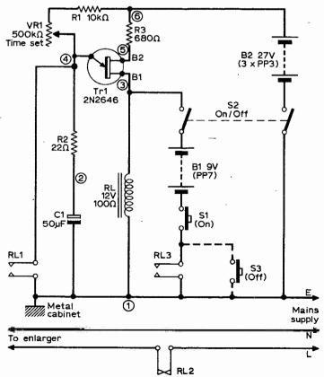
Fig. 10: Photographic enlarger timer. Pressing S1 de-energises the relay for a time set by VR1. While the relay is de-energised the enlarger is on.
