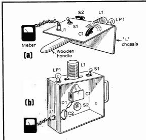
Fig. 2: (a) suggested method of construction using an L-shaped chassis.
