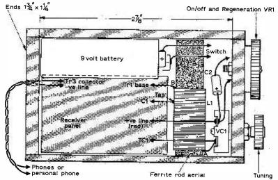
Fig. 4: Case dimensions and general assembly.
