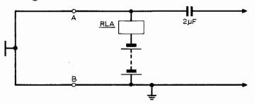
Fig. 8: When the handset is lifted G1 and G2 (Fig. 6) close operating relay RLA at the exchange.
