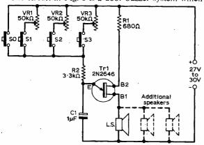
Fig. 7: Multitone calling system. VR1–VR3 are adjusted to give different pitched buzzes.
