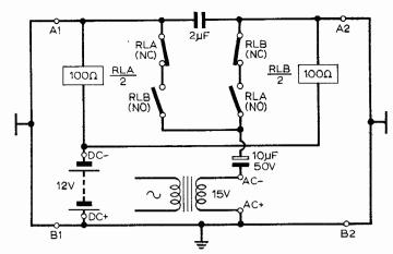
Fig. 9: Circuit for two-way communication using a pair of standard desk telephones.
