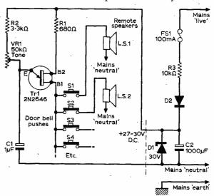
Fig. 8: Multispeaker buzzer system. Note importance of safety precautions in text if using the non-isolated power supply shown.
