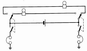
Fig. 3: A further modification, using a bell calling system.
