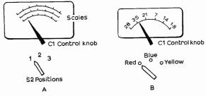
Fig. 3: (a) method of calibration if general coverage calibration is required. A scale arc is provided for each of the three positions of S2 and is calibrated at (say) 500kc/s intervals.
