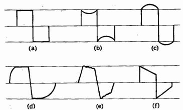
Fig. 4: Square-wave testing of amplifier: (a) square-wave input, (b) low frequency loss, (c) low-frequency boosted, (d) high frequency roll-off, (e) high frequency boosting causes ringing, (f) low-frequency phase shift.
