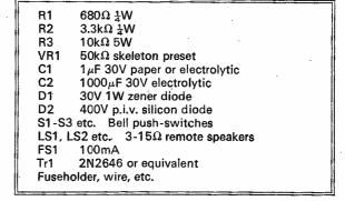
this was a permanent installation a very simple non-isolated power supply was used. Capacitor C2 is trickle charged through R3 and D2 up to a potential of 30V when the zener diode conducts away further current. If this power supply is used it *must* be connected to the mains with the polarity as shown or the wiring will become dangerously "live".
