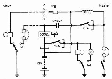
Fig. 5: Practical circuit based on the system shown in Fig. 4 and incorporating a relay ringing system. This arrangement requires an operator or master station.
