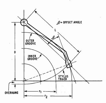
Fig. 1: Pick-up arm constants—horizontal plane.
