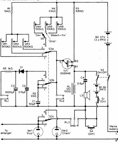
Fig. 12: Colour photographic timer. S3 settings: (1) Red exposure, set by VR1; (2) green exposure, set by VR2; (3) blue, exposure, set by VR3; (4) audible chemical bath time warning, three different preset periods set by S5.
