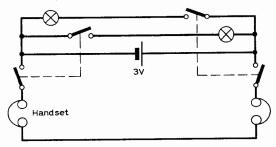
Fig. 2: Practical version of the previous circuit using a lamp calling system operated by switches.
