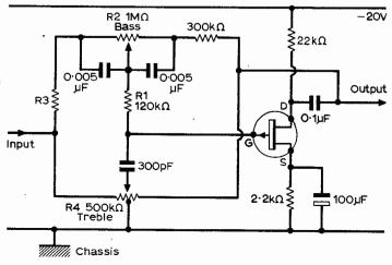
Fig. 5: A p-channel JGFET in a Baxandall tone control circuit.
