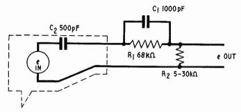
Fig. 7: Matching network for constant amplitude cartridge into pre-amp with constant velocity equalisation.
