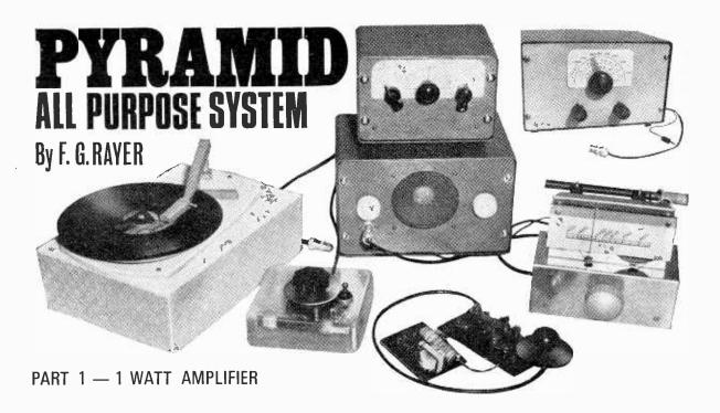
HIS set of equipment consists of a high-gain 4-transistor amplifier, with battery and loud-speaker, into which can be plugged various accessory units. A very versatile set of equipment is thus easily built up, according to the user's needs.
