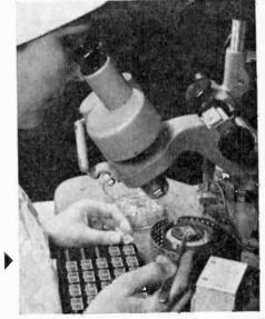
Bonding a silicon integrated circuit chip into a \(\frac{1}{4}\)" \times \(\frac{1}{8}\)" flat pack.
