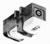
Goldring Manufacturing Co. (GB) Ltd., 486–488 High Road, Leytonstone, London, E.11, announce their new stereo magnetic cartridge, No. 800. In this unit, a very lightweight tube of magnetic material lies in a "free field" generated by a fixed source and is made to follow the record groove modulation by its
