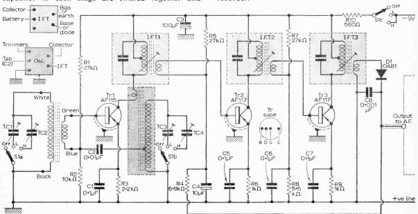
Fig. 2: Circuit diagram of the mixer, two i.f. amplifiers and the detector.
