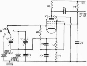
Fig. 3: Original "lash-up" of the crystal oscillator stage.
