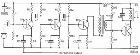
Fig. 1: Circuit diagram of the complete VOX unit.
