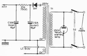
Fig. 2: Circuit of the power supply system.
