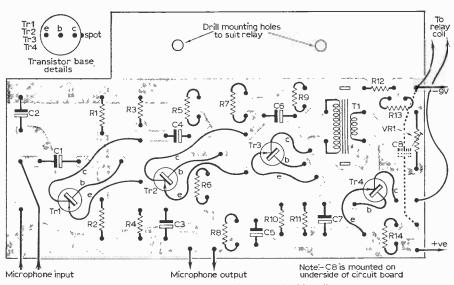
Fig. 2: Printed circuit board layout and wiring diagram.
