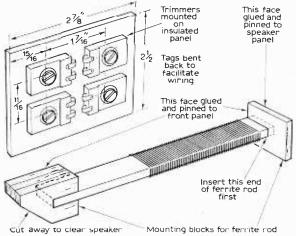
Fig. 4: Details of the ferrite rod and trimmers.
