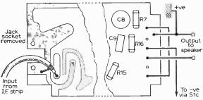
Fig. 5: Connections to the pre-wired audio amplifier.
