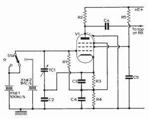
Fig. 4: Oscillator circuit with only one crystal tuned.
