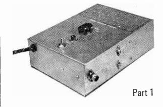
EXT to the multimeter, a good crystal calibration oscillator is probably one of the most useful pieces of test gear to the radio enthusiast. Apart from its obvious use in calibrating receivers, it can also be used to calibrate or check the calibration of v.f.o.s, signal generators, g.d.o.s, absorption wavemeters, etc. Furthermore, since the frequency of the signals it generates is to all intents and purposes constant, it can be used to detect and estimate
