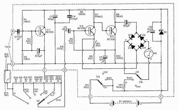
Fig. 1: Circuit diagram of the a.c. millivoltmeter.
