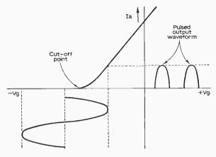
Fig. 5: Class C valve operation.
