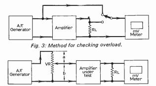
Fig. 4: Simple attenuator to assist users of unknown test equipment.
