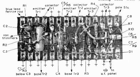
A circuit diagram is provided with each board so there should be no problems. The input is taken to C1 on this circuit, and the output taken direct from C7, C4 is shorted to the slider of RV2 as advised above.
