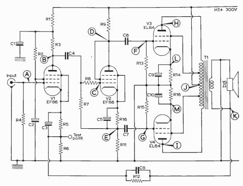
Fig. 1: Typical audio amplifier with suggested test points.
