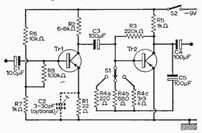
Fig. 5 (above): Circuit diagram of the preamp. Fig. 6 (right): Veroboard layout and wiring.
