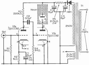
Fig. 1: Circuit of the transmitter.
