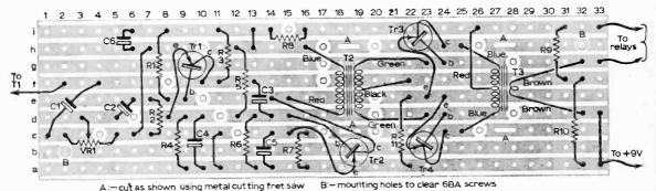
Fig. 3: Component layout diagram, showing theoretical components upon the Veroboard. In fact, all components are vertically mounted on the board to save space. One must be careful about the colour coding of the transformers T2 and T3, since the coding may only hold true for the types specified in the components list.
