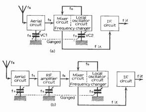
Fig. 1: (above) (a) Block diagram of superhet front-end less r.f. stage. (b) front-end block diagram with r.f. stage. fs is signal frequency, fo oscillator frequency and f.i.f. is the intermediate frequency.
