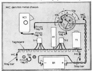
Fig. 5: Rear of panel layout and wiring.
