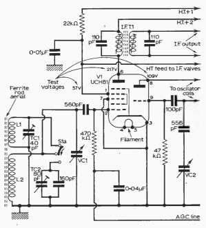
Fig. 4: The front-end section of a battery portable, L1 and L2 being the ferrite rod aerial.
