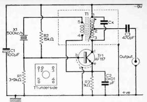
Fig. 2: Alternative circuit for the Crystal Oscillator.
