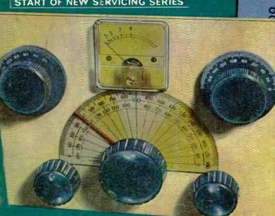
**MULTIBAND** TRANSISTOR SUPERHET
