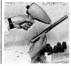
This instrument is a fully portable electroplating "gun". It comes in a kit which consists of 'Plectro' gun, and nine separate cartridges for plating gold, silver, brass, tin, cadmium, zinc, copper, nickel and chromium. The gun is powered by its own self-contained battery, but very large areas of plating can be tackled by using a suitable accumulator.
