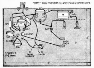
Fig. 3 (above): Layout of the prototype (Fig. 1).
