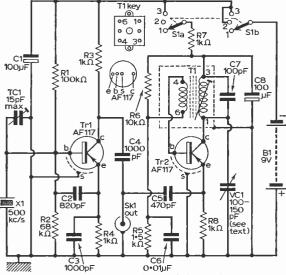
Fig. 1; Complete circuit of the marker.
