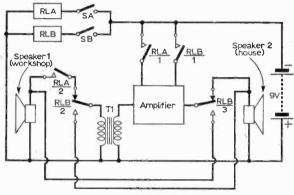
Fig. 1: Block schematic diagram of the complete intercom. Note how the relays are used to switch the speakers so that either one can be used as a microphone.
