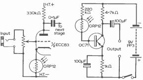
Fig. 2a: Valve receiver circuit.
