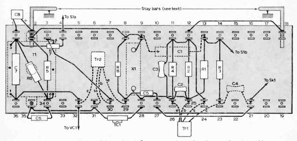
Fig. 3: Layout and wiring of the tag board. Components shown dotted are on the reserve side.
