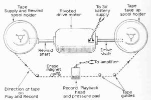
Fig. 1: Basic arrangement of tape transport system.
