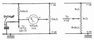
Fig. 5: Details for wiring in an "S" meter. The diagram on the right shows an alternative to the  $10k\Omega$  pot.
