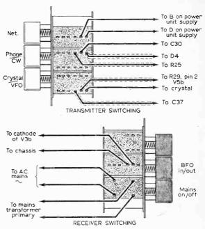
Fig. 6: Wiring details of the push-button units.
