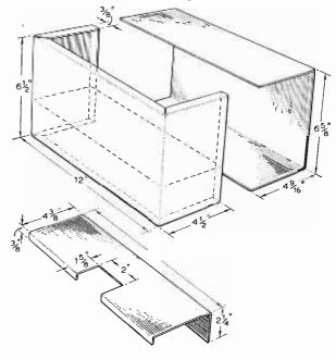
Fig. 7: Size and constructional details of the case.
