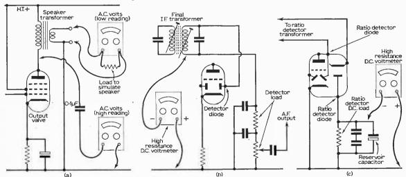
Fig. 3: Output monitoring arrangements. (a) monitoring the a.f. with the generator input signal modulated, (b) monitoring the detector load voltage on unmodulated carrier output and (c) monitoring the voltage across the d.c. load of an f.m. radio detector.
