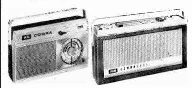
The latest in the K-B range of portable radios are the Cobra (left) and Commodore (right). Both models feature modular construction which makes servicing a very easy job—the r.f., i.f. and a.f. sections being three plug-in units. The transistor complement is the same in both receivers: 2 × AF117, OC70, 2 × AC127 and 2 × OC81.
