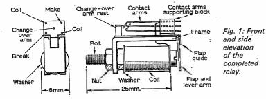
If one was to use a material with permanent magnet properties, the contacts would permanently remain in the energised position.
