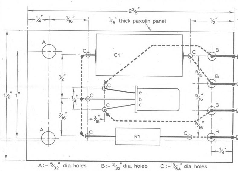
Underside wiring of paxolin panel is 15A fuse wire (shown dotted)
