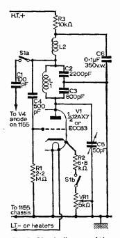
Fig. 2: Circuit diagram of the "Q" Multiplier.
