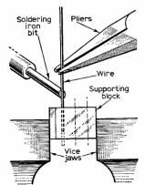
Fig. 9: (left) Method of locking wire contact arms in supporting block.
