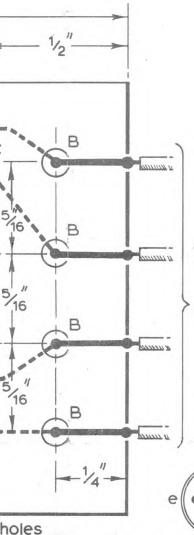
Flexible leads to the other components. These are secured by 3/4" of the core being bared, threaded through (as shown) and soldered
