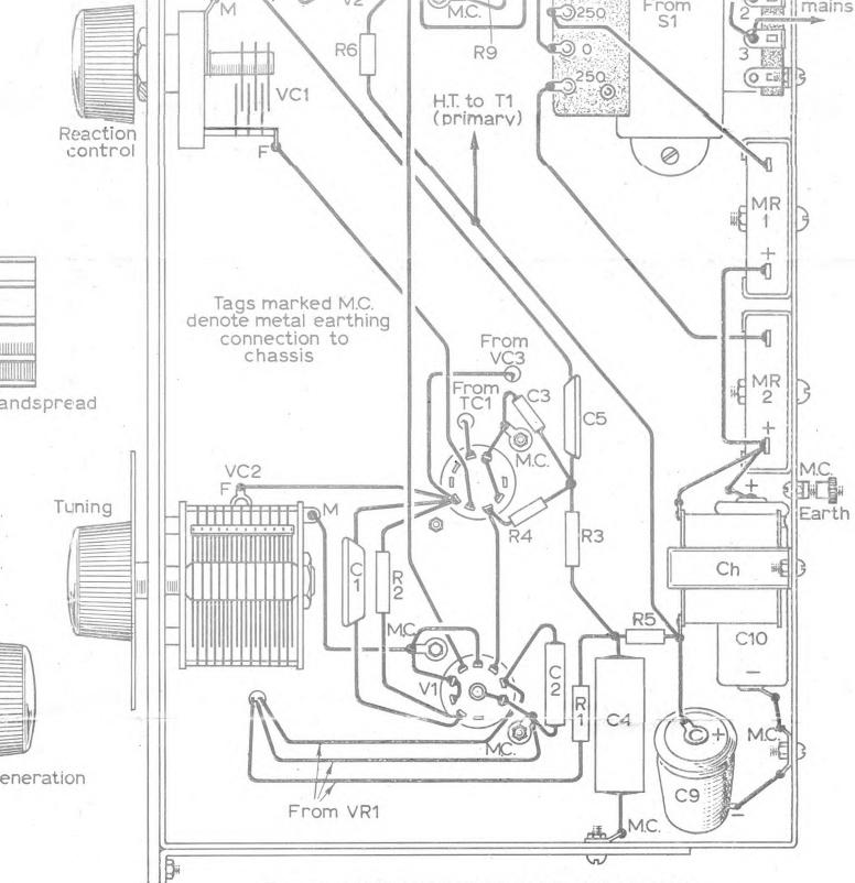
Fig. 3 UNDERSIDE OF CHASSIS
