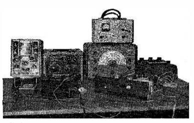
Fig. 9. Stereo tuner undergoing oscilloscope/wobbulator alignment.
