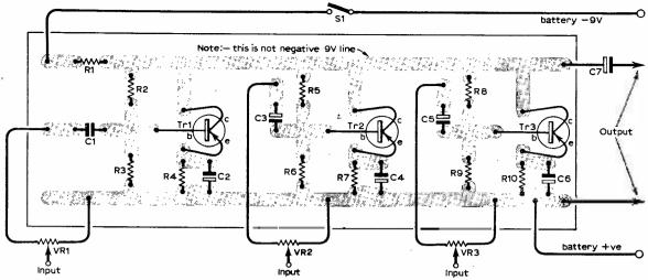
type, input 1 was designed for use with high-impedance sources, such as record decks or crystal microphones. The other inputs are low impedance, for use with dynamic, moving-coil or magnetic mikes.
