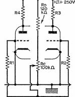
Fig. 1: Modifications to the gating oscillator VI to give continuous coverage from 50c/s to 5kc/s.
