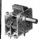
Designed for use in miniature transistor receivers. The front (aerial) section is 208pF to provide coverage for medium waves. and the rear section is 176pF, which may be padded to match the oscillator—very robust yet lightweight. Front area  $1\frac{3}{8}$ in. x  $1\frac{17}{32}$ in. x 1in. deep. PRICE 12/6.
