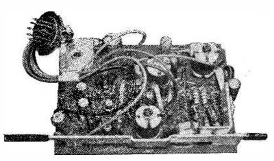
Fig. 6. Commercial stereo decoder unit designed for plugging into the Bang and Olufsen Beomaster 1000, integrated stereo tuner and hi-fi amplifier.
