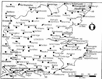
Wrotham and Swingate are the only two BBC sound stations to radiate stereo. The contours on the map indicate field-strength in dB relative to  $1\mu V/m$  for a receiving aerial height of 30 ft.
