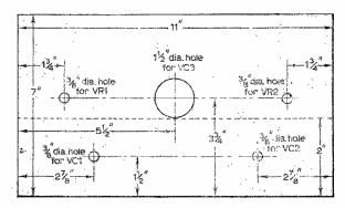
Fig. 4: Dimensional data for the front panel. If one does not have a cutter large enough to tackle the hole for VC3, drill a lot of smaller holes just inside its circumference, then break away the unwanted metal and finish the job off with a file.
