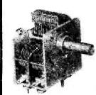
"00" Twin Condenser Designed for use in miniature transistor receivers. The front (aerial) section is 208pF to provide coverage for medium waves, and the rear section is 176pF, which may be padded to match the oscillator-very robust yet lightweight. Front area  $1_{\frac{3}{4}}^{\frac{3}{4}}$ in. x  $1_{\frac{1}{3}}^{\frac{1}{2}}$ in. x  $1_{\frac{1}{3}}^{\frac{1}{2}}$ in.
