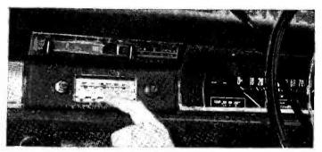
Grundig (GB) Ltd., announce the AS40 car radio. It has long, medium and short wave (49 metre bandspread) and v.h.f. wavebands with an efficient switchable a.f.c. circuit ensuring crystal clear reception on v.h.f. Waveband selection is by simple press-button control and a speech/music control is also provided. It can be powered by either a 6V or 12V car battery and is fitted with a lead for connection of multiple loudspeakers.
