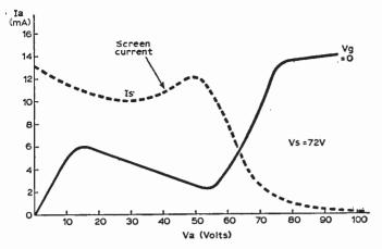
Fig. 62t Ia/Va curve for a tetrode. (Screen current against screen voltage shown dotted.)
