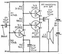
Fig. 1: The three-transistor, transformerless circuit of the amplifier.
