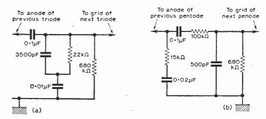
Fig. 10: Record equalisation arrangements for preamplifiers with (a) triode circuits and (b) pentode circuits.
