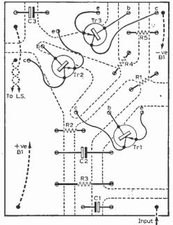
Fig. 3: The layout of components on the plain side of the board. The actual size of the board is lin. x 13 in.
