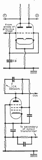
Fig. 9: An input stage of an amplifier in which a CR network in the anode circuit helps stability at high frequencies.
