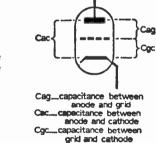
Fig. 59: Interelectrode capacitances in the triode valve.
