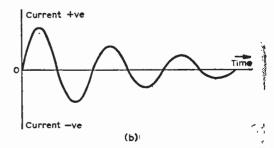
Fig. 64: (a) Discharging a capacitance through a coil; (b) damped oscillations.,
