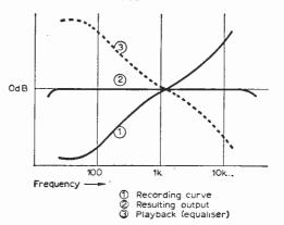
Fig. 10 (c): Illustrating graphically the action and effect of record equalisation.
