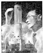
This STC technician's task (left) is a delicate one. He is lining up the cage grid of a powerful radio broadcast valve which has been manufactured at the Paignton works of Standard Telephones and Cables Limited.
