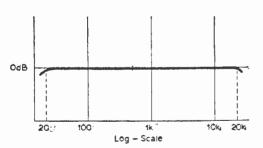
Fig. 1: A frequency response graph. The horizontal scale is measured in cycles per second (c/s).
