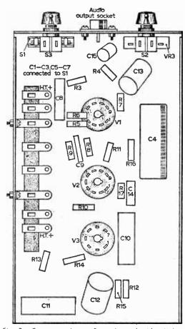
Fig. 3: Component layout from the underside. Valveholder spigots should be taken to chassis. VRI, 2, RI, R2 are above the chassis.
