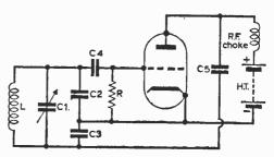
Fig. 66: (c) The Colpitts oscillator.
