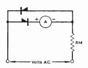
Fig. 2: An alternative half-wave rectifier voltmeter.
