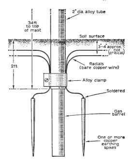
Fig. 2: Details of the base of the mast, buried below ground with all its earthing attachments.
