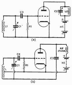
Fig. 66: (a) A tuned-anode, tuned-grid oscillator; (b)
