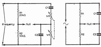
Fig. 4a (left): The frequency measuring circuit VR is a Im  $\Omega$  twin-gang log. potentiometer. Fig. 4b (right): The bridge circuit.
