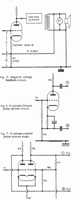
hence the total input now required for full output would be that required for full output without feedback plus 2.3V. The feedback ratio is Vi/Vii.
