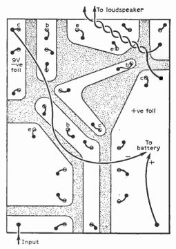
Fig. 2: The layout for the printed circuit. The shaded portions are etched clean of the copper.
