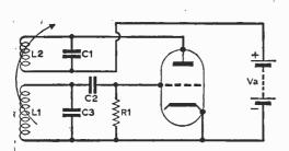
Fig. 65: A simple oscillator circuit.
