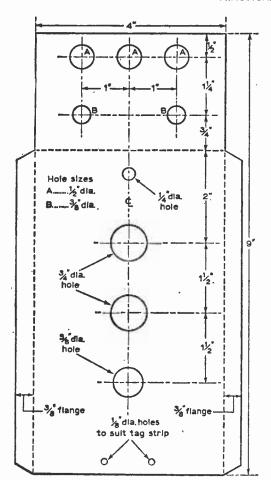
Fig. 2t Drilling layout for the audio oscillator chassis.
