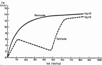
Fig. 63: Ia/Va curve for a pentode. (Same curve for tetrode shown dotted for combarison.)
