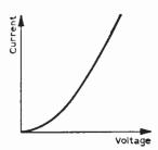
Fig. 3: The characteristic curve for a typical rectifier.
