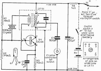
Fig. 5: A transistorised crystal frequency marker circuit which can be used to calibrate the "Ten-Five" accurately. I.F.T.I. is a Denco sub-miniature i.f. transformer, type IFT14. C2 is a 6v d.c. working component.
