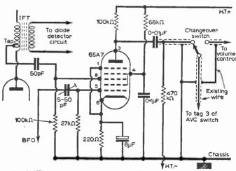
Fig. 2: The circuit arrangement as used by the author in the R1155.
