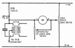
Fig. 1: An alternative 'S' meter circuit.
