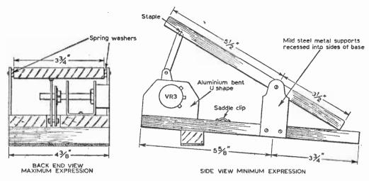
Fig. 15: Construction details of the expression pedal.
