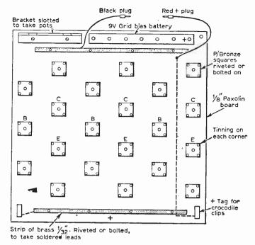
Fig. 16: The quick "hook-up" board as used by the author.
