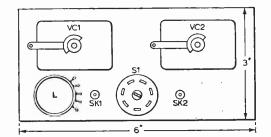
Fig. 4: The circuit of Fig. 3 may be constructed as a compact unit using the above layout.
