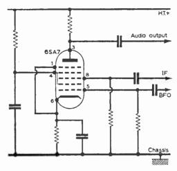
Fig. 1: The basic product detector circuit.
