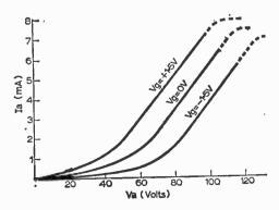
Fig. 53: A typical family of la/Va curves for a triode, with grid voltage (Vg) kept constant.
