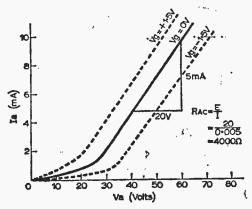
Fig. 54: Obtaining a triode a.c. resistance on the  $l_a/V_a$  graph at  $V_g = 0$ .
