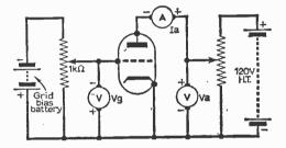
Fig. 52: The circuit arrangement used to determine the current/voltage curve (la/Va) for a triode.
