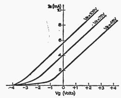
Fig. 551 A set of mutual characteristics curve of a triode.
