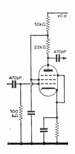
For wide-band amplification at kilocycle frequencies r.c. coupled i.f. stages are as good as heavily damped tuned circuits and permit simple the cheap arrangement shown in Fig. 1 V4). (V3. saving of the cost of i.f. transformers justifies the use of two double triodes я four-stage amplifier that provides enough gain for any reasonable reception area. Valve for valve. double triodes give more gain than single pentodes.
