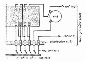
Fig. 13: Details of the tuning resistance strip.
