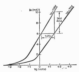
Fig. 57: Obtaining the amplification factor of a triode.
