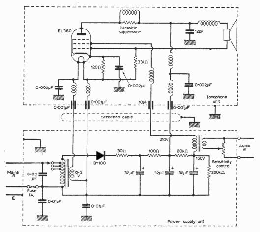
Fig. 1: The basic circuit of the lonophone loudspeaker system.
