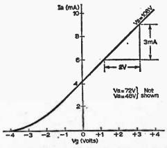
Fig. 56: Obtaining the mutual conductance of a triode.
