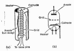
Fig. 51 (a): The mechanical construction of a triode, without the glass envelope. (b): The triode valve circuit symbol.
