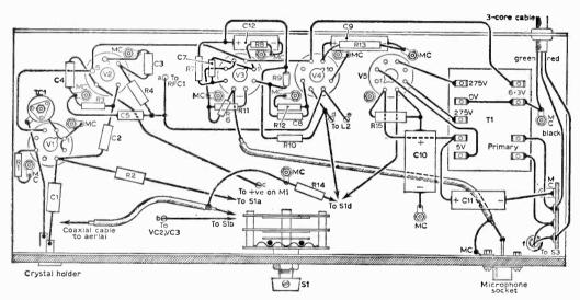
Fig. 3: The underchassis wiring of the transmitter.
