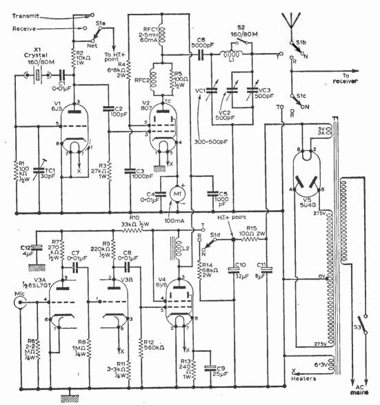
fig. 1: The complete circuit of the transmitter.
