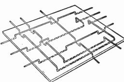
Fig. 1: The method of "stitching" connecting wires between holes made in a paxolin chassis.
