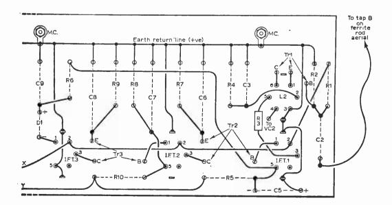
Fig. 3b: The wiring; mixer, i.f. and detector.
