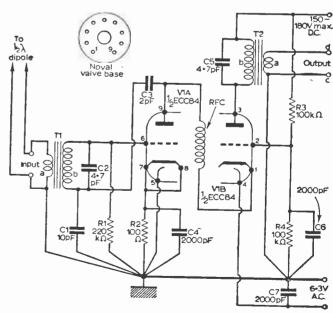
Fig. 3: The circuit of Unit "A", the signal preamblifier.
