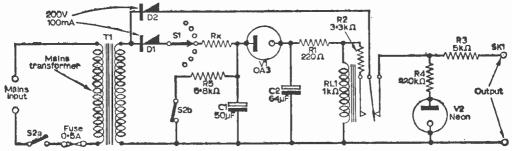
Fig. 1: In this circuit of the timer unit, all switches are shown in the "unit off" position.
