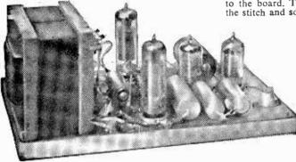
amplifier constructed by the author which shows the clean layout obtainable using bread-board wiring.
