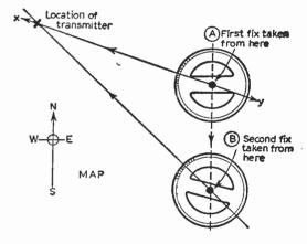
Fig. 8: Another typical direction finding arrangement.
