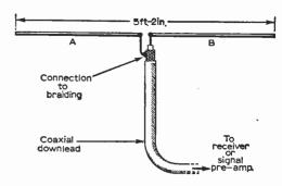
Fig. 91 The dimensions and connections of a v.h.f./f.m. dipole.
