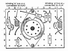
Fig. 51 Wiring of Unit "A" on the plain side.
