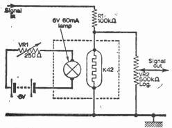
Fig. 11: A practical remote volume control circuit.
