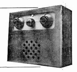
THIS receiver is designed to avoid the difficulties which often arise in aligning aerial and oscillator stages. It is usual to employ a ganged capacitor for aerial and oscillator tuning and efficiency falls off badly if tracking of these circuits is not correct.
