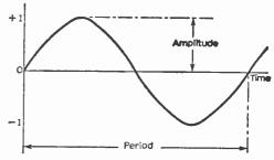
Fig. 25: An a.c. waveform.
