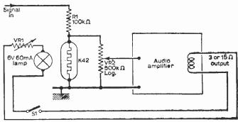
Fig. 14: A volume compressor for variable output levels.
