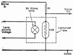
Fig. 10: The basic circuit of a light-operated volume control.
