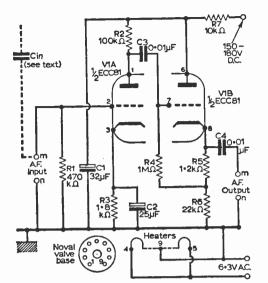
points are at low impedance. In this section the load resistor is R6 in the cathode circuit, R5 merely being a bias fixing item.
