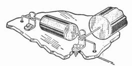
Fig. 2: Methods of anchoring components to the panel.
