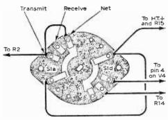
Fig. 4: Connections to the switch, SI.
