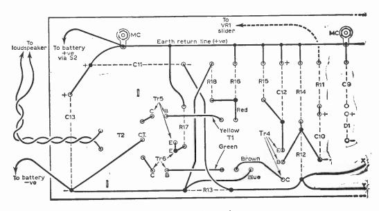
Fig. 3a: The underside wiring: driver and output stages.
