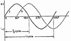
Fig. 26: Phase differences in alternating currents.
