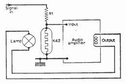
Fig. 13: A volume compressor circuit.
