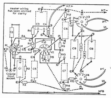
Fig. 4: The bread-board wiring diagram of the amplifier circuit of Fig. 3.
