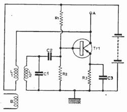
Fig. 30: Circuit of an LC oscillator. CI prevents the base ifrom shorting to earth.
