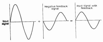
Fig. 26: The input signal with negative feedback applied.
