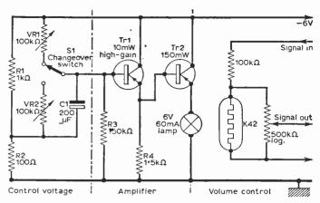
Fig. 15: A circuit for automatic attack/decay control.
