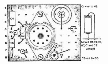
Fig. 7: Wiring of Unit "B" shown from the conductor side.
