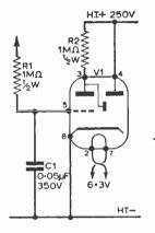
The grid is connected to the a.v.c. line in an a.m. receiver; or to the negative end of the discriminator stabilising capacitor in an f.m. receiver.
