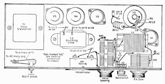
Fig. 2: The above-chassis layout of components.
