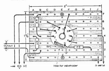
Fig. 4: Wiring of Unit "A" shown from the conductor side.
