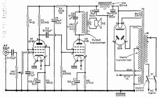
Fig. 7: The circuit of an inexpensive signal tracer.
