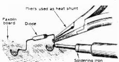
Fig. 5: Using a pair of pliers as a heat shunt during soldering.
