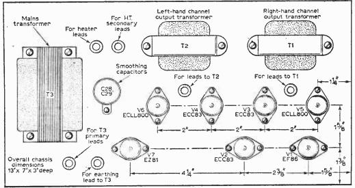
Fig. 3: Above-chassis layout and dimensions.
