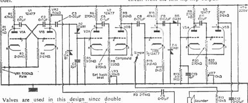
Valves are used in this design since double triodes were then, and possibly still are, cheaper than a pair of reliable transistors. However, the principle could be extended to transistor circuitry if required.
