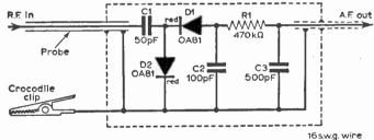
Fig. 4 (above): The circuit of the diode probe unit.
