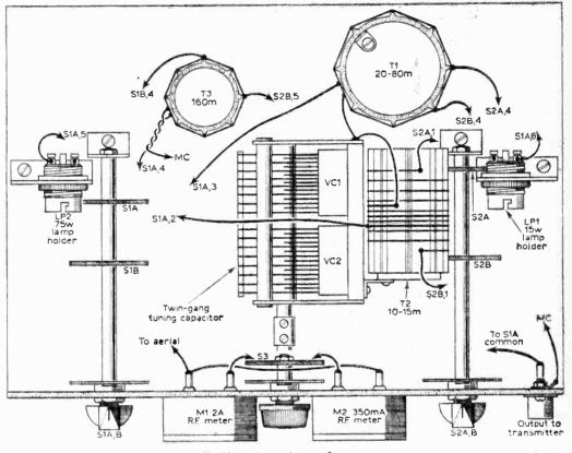
Fig. 2: Above-chassis layout of components.
