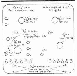
Fig. 1: Drilling details of the plastic board.
