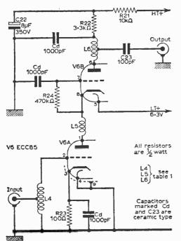
Fig. 2: The circuit of the pre-amplifier for 144Mc/s and 190Mc/s.
