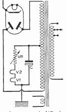
then passes through the heaters and VR is adjusted to provide the correct energising current. The centre-tap is thus negative to chassis. This negative voltage may also be used as a convenient source of bias. The electrolytic capacitor C will invariably be found and acts as a bypass to the low frequencies and as a bias filter component.
