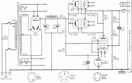
Fig. 1: The circuit diagram of the power pack.
