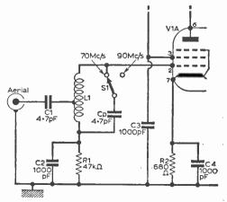
Fig. 1: The modified circuitry of VI (see Fig. 1, page 220 of the July 1963 issue).
