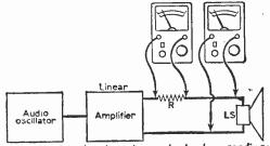
Fig. 6: Loudspeaker impedance check. Low readings only.
