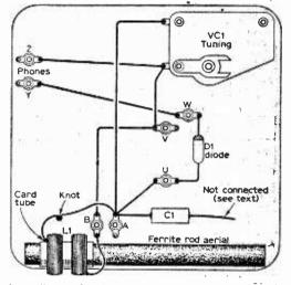
the coils coming loose. The knotted wire is: "A," in Fig. 3, the unknotted end being "B". If the coil has been correctly wound the ferrite rod will slip nicely in and out of the coil at will.
