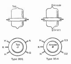
Fig. 4: Connections to two types of acorn valves which may be used in this set.
