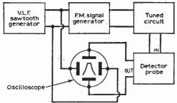
Fig. 8a (above): Using the probe in conjunction with an oscilloscope.
