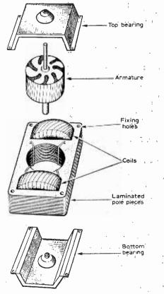
Fig. 1: The construction of an induction motor.
