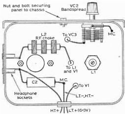
Fig. 3a (above): The underside wiring; b (below) t the wiring on the top of the chassis.
