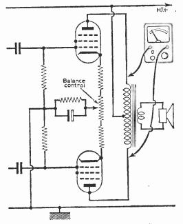
Fig. 5: Push-pull output stage balance adjustment.
