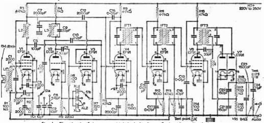
Fig. 1: The circuit of the tuner which includes Foster-Seeley phase discriminator.
