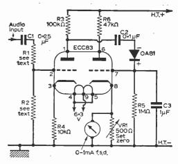
Fig. 3: The recording level meter circuit as used by the author
