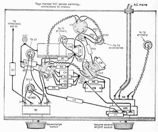
Fig. 3: The underchassis wiring diagram.
