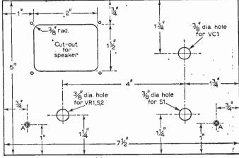
Countersunk holes marked 'A' are for bolts securing panel to chassis
