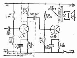
Fig. 4: Class A output stage with R-C coupling.
