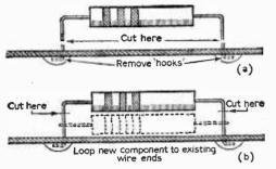
Fig. 5a and b: How components are soldered on to printed circuit boards.
