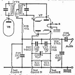
Fig. 2: The alternative ratio detector stage.
