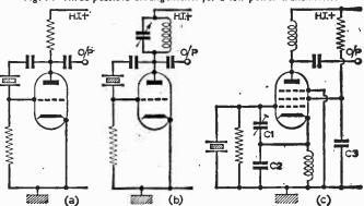
Fig. 8: Crystal oscillator circuits.
