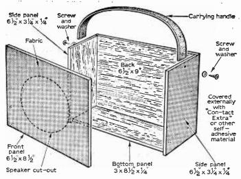
Fig. 6: Construction details of the cabinet.
