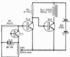
When the temperature of the sensing transistor Tr1 rises, the base of Tr2 becomes negative, consequently the collector current rises, causing the negative voltage applied to the base of Tr3 to fall. The resultant fall in the collector current of Tr3 causes the relay RL1 to de-energise, so breaking the circuit to the heater.
