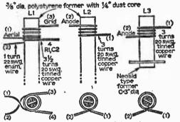
Fig. 6: Winding details of the coils.
