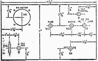
Fig. 10: Details of the front panel.
