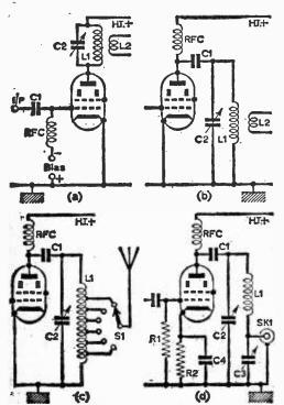
Fig. 9: Various power amplifier stages.
