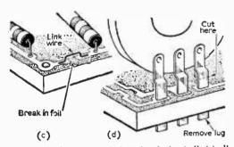
Fig. 5c: Bridging a crack in printed circuit "wiring". Fig. 5d: Removing a tagged component from a printed circuit board.
