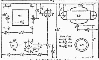
Fig. 11: The layout of the chassis.
