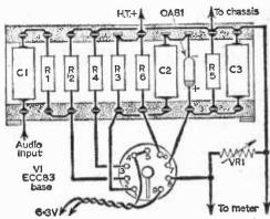
Fig. 4 Wiring diagram of the circuit of Fig. 3.
