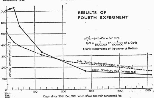
Fig. 1: Actual results for radioactivity and its decay with time, for a pair of typical rain and snow samples.
