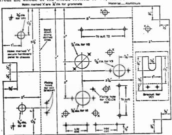
Fig. 2: Chassis dimensions and drilling details.
