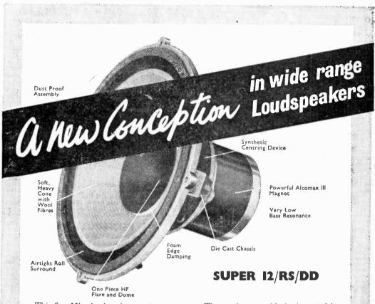
This fine 12in. loudspeaker employs a new type of double diaphragm assembly (patent application No. 40667/60). The main cone is moulded from a specially formulated soft pulp which reduces break-up effects to a minimum. Higher frequencies are radiated by a one piece tweeter cone with its edge supported on foam plastic to avoid resonance.
