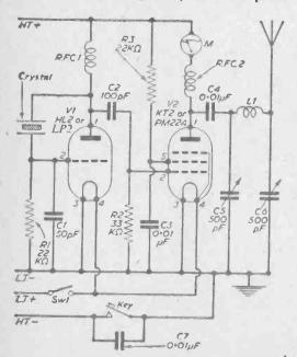
amplifier valves are connected in parallel, power can be raised to 2.5W. That this power is sufficient can be shown by the fact that within half an hour of going on the air for the first time with the set, contacts had been made from the east coast with North Wales, South Wales and France, all on 7Mc/s.
