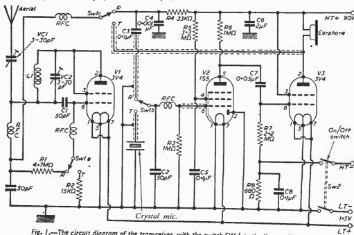
Fig. 1.—The circuit diagram of the transceiver, with the switch SW.1 in the "receive" position.
