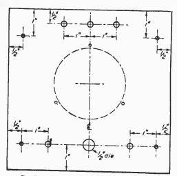
Fig. 2.—The drilling details of the panel.
