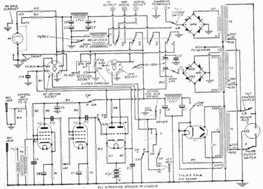
Fig. 1.—The circuit of the modulator and power unit.
