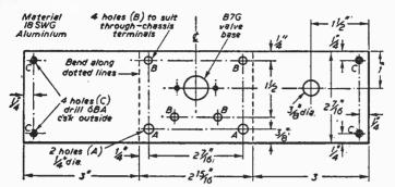
Fig. 5.—Drilling details of the oscillator chassis.
