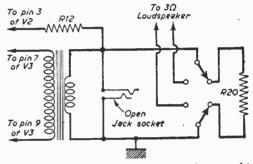
Fig. 14.—The circuitry of the output transformer and its associated components.
