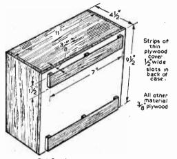
Fig. 5.—A rear view of the case.
