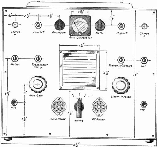
Fig. 2.—The layout for the panel of the modulator and power unit.
