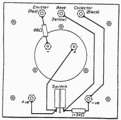
Fig. 4.—The wiring details.
