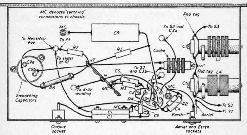
Fig. 3.—The under-chassis wiring diagram.
