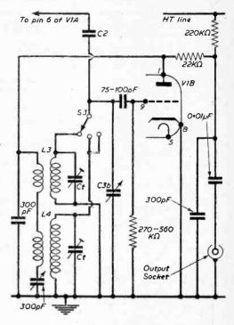
Fig. 5.—Alternative circuitry to give improved gain and overall sensitivity.
