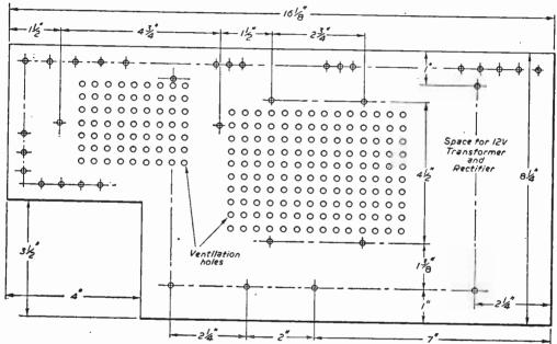
Fig. 5.—Details of the rectifier support.
