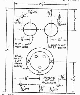
Fig. 18 (Above).—The drilling dimensions for the mains input panel.
