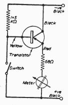
Fig. 3 (Left).—The circuit of the tester.
