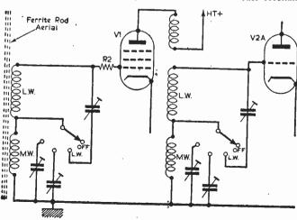
Fig. 6.—A possible modification for receiving one L.W. station.
