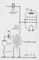
different values of inductance will be required in the 1.1 position. These various values may obtained by having sufficient inductance for the lowest frequency upon which the transmitter will be used and then when operating on the higher frequency bands, short out-by means of a switch, or flexible link wanted portions of the inductance. Handy though either method
