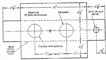
Fig. 2.—Constructional details of the main case.
