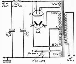
Fig. 2.—Circuit diagram of the power supply.
