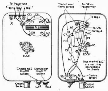
Figs. 5 and 6 (left and right).—Above— and below—chassis wiring of the A.F. modulator. Another valveholder—for V5—should be mounted on the chassis at point X with the same orientation as the holder for V2.
