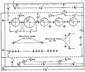
Fig. 3 (Above).—The constructional details of the modulator sub-chassis.
