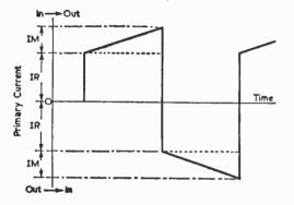
Fig. 2 (above).—The trapezium shaped current waveform.
