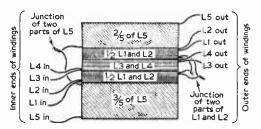
L1 and L2....45 turns each L3 and L4....8 turns each L5......500 turns total Fig. 4.—A section through the transformer windings.
