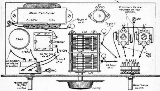
Fig. 2.—The above-chassis layout and wiring details.
