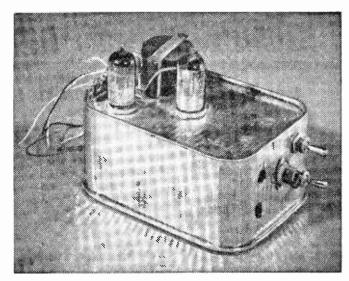
The audio modulator section (showing V5 in position, also)
