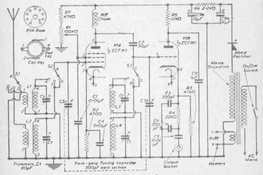
Fig. 1 .- The circuit of the Tuner.
