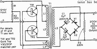
Fig. 1.-The circuit of the inverter.
