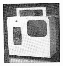
field strength for both the medium-wave Home and Light programmes of the BBC and so, with the economic considerations in mind, a TRF circuit with switched tuning was chosen.
