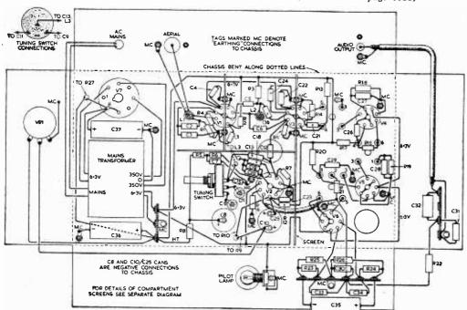
Fig. 3.—Underchassis component layout and wiring diagram.
