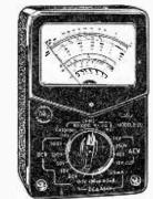
MODEL A-10 (500 Micro-amp Movemodel A-III (300 Micro-amp Movement). D.C. (2k per volt) 0/10/50/250/500/1000 v. A.C. (2k per volt) 0/10/50/25/25/25/500/1000 v. D.C. current 0/0.5/25/250 mA. Resistance: O/10K/1 Meg. Size: 5½ x 3½ x 1½in. Weight: 17 ozs. Price £4.17.6, P.P. 1/6 inclusive of Test Prods, Instruction Book and Batteries
