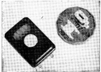
A miniature microphone and two polystyrene coil formers.
