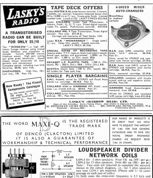
In both cases the cross-over frequency is 2.5 kc/s and with the constant resistance circuit recommended, the attenuation beyond the cross-over frequency will be 12 dbs per octave.
