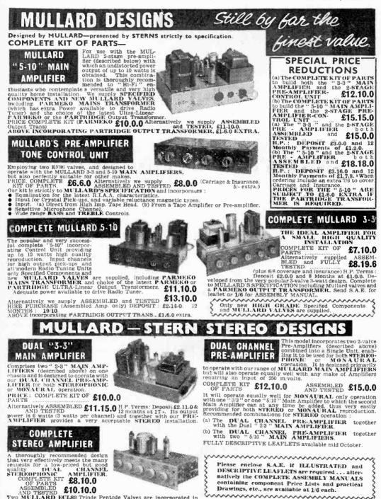
ASSEMBLED £10.10.0 AND TESTED TETTED £10.10.0 Two MULLARD ECL92 Triode Pentode Valves are incorporated in the design : they form a "CLASS A" single-ended output stage in each channel. The input sensitivity is 300 m/volts, therefore when used with most STERIO Crystal Pick-Ups, or Radio Tuning Units, en output of 2 watts per channel is achieved, or similarly when switched to MONAURAL Pick-Up position a combined output of 4 watts is produced.
