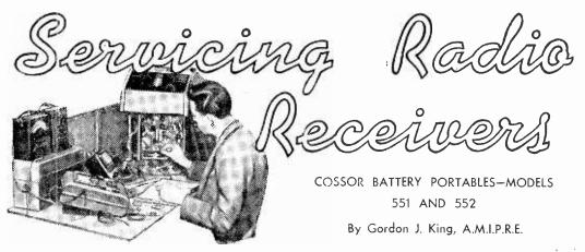
BOTH these models feature four valves of the low-consumption all-dry range and almost identical circuits. Model 551 is a small cabinet version with the controls mounted on the top, while Model 552 takes the form of an attaché case. The cabinets are covered with a Lionide material and a substantial handle is featured for ease of carrying.
