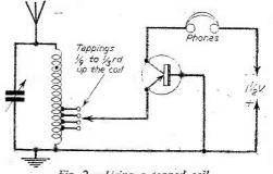
Fig. 2.-Using a tapped coil.
