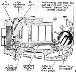
Fig. 6.—Rear of chassis after conversion.
