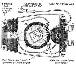
Fig. 2.—Inside front of case after construction of diode receiver.
