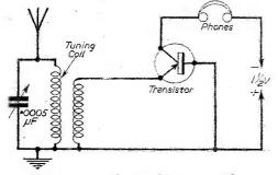
Fig. 1.-Transistor as detector-amplifier.
