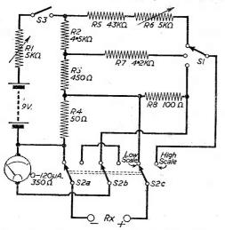
Fig. 10.—An ohmmeter circuit with four ranges which provides measurement between  $1\Omega$  and  $2 M\Omega$ . The lowest range has a separate scale.
