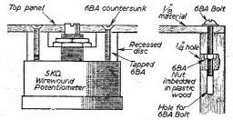
Fig. 8.—An unobtrusive method of mounting the pre-set potentiometers.
