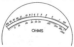
Fig. 12.—The two scales of the olummeter of Fig. 10. Mid-scale readings 5 (x 100, etc.) and  $45\Omega$ . The upper scale is for the three series ranges ; the lower scale is for the lowest range, which uses the shunt method.
