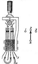
Fig. 11.—Connecting up a three-position key switch as one-pole, threeway.
