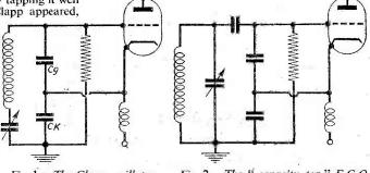
Fig. 1.—The Clapp oscillator.
