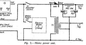
motor panel in any convenient position (see Fig. 1), provided the filament transformer is not underneath the pick-up when it is on a record. The L.T. of 6.3 volts is taken from a small filament transformer, although the writer used a large speaker transformer, which gave just under 6 volts on load with 240 volts mains fed into the old anode windings. The thick
