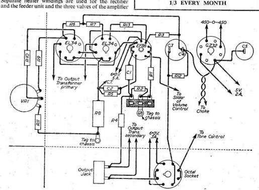
Fig. 16.-Wiring diagram of the 20-watt model.
