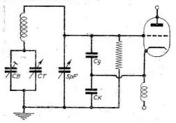
Fig. 9.—A 5 pF condenser connected as shown gives a "velvet vernier" control of a few Kc/s frequency shift in the Clapp V.F.O. circuit. CB is the "bandsetter." CT is the usual tuning control.
