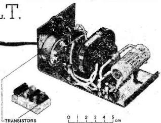
Converters with 2mW and 4 to 6W output.
