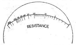
Fig. 4.—Scale of the ohmmeters of Figs. 2 and 3. Mid-scale value=15. On the different ranges the figures are to be multiplied by factors of 100, 1,000 and 10,000 respectively to give ohms values.
