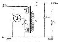
Basic circuit of ringing choke converter.
