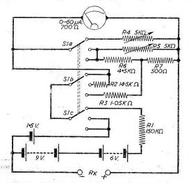
Fig. 3.—Circuit of an ohmmeter covering  $100\Omega$  to 5  $M\Omega$  in three ranges with a common scale.
