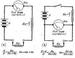
Where D = Full Scale Deflection. (i.e. with Rx = 0 and  $\infty$ ) d = Deflection with Rx (from left side)<math>Ro = Value of Rx for half-scale deflection<math>D-d = Deflection with Rx (from right side)
