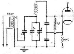
Fig. 10.—Between transmissions V.F.O. drift may be minimised by using a relay to switch in a detuning capacitor (CS). This shifts the V.F.O. frequency outside the band, but the V.F.O. valve still oscillates and therefore does not cool off during stand-by periods. After initial warming up the V.F.O. frequency during transmission becomes stable.
