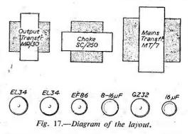
the 1,000-ohm cathode resistor directly under the hole in the chassis where the wires are taken through. This will assist in ventilation, as nearly 20 watts of heat has to be radiated away.
