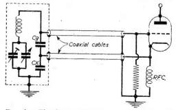
Fig. 4.—The "remotely tuned" Clapp V.F.O. The tuned circuit may be separated from the transmitter by using several feet of coaxial cable as shown. The tuned circuit is preferably enclosed in a screening metal case, thus giving "table top" control of frequency.
