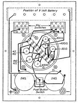
Fig. 7.—The reverse of the top panel, showing the components and some of the wiring.
