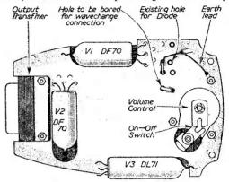
Fig. 3.-Rear of chassis after conversion.
