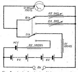
Fig. 2.—A simple circuit which measures from  $1 \ K\Omega$  to  $5 \ M\Omega$  in two ranges. Maximum current approximately 100µA. A single scale serves for both ranges.
