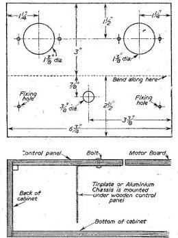
Fig. 4.—Details of the chassis—tinplate or aluminium.
