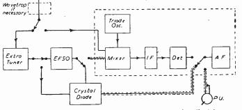
Fig. 1.-Schematic diagram of the arrangement described here.
