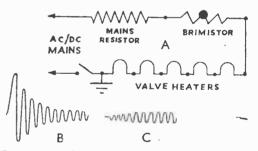
Diagram " A " shows the correct positioning of a Brimistor in the average circuit.
