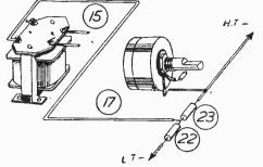
Fig. 23.—Pictorial diagram of the auto-bias wiring,
