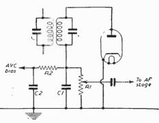
Fig. 1.-Simple diode detector and A.V.C. circuit.
