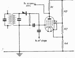
Fig. 2.—Circuit of diode detector and control valve for supplying A.V.C. to screen grids for improved control.
