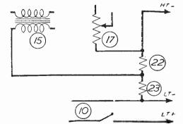
Fig. 22.—Modified circuit for providing automatic grid bias.
