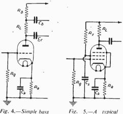
Fig. 4.—Simple bass compensation circuit.
