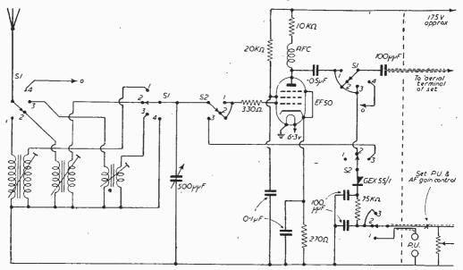
Fig. 2.—Theoretical circuit of the amplifier or R.F. stage.
