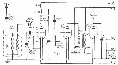
Fig. 1.—Theoretical circuit of the receiver.
