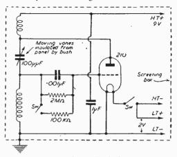
Fig. 2.—Simple oscillator circuit for test purposes.
