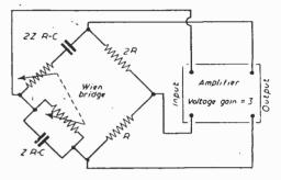
Fig. 1.-Theoretical set-up for using the bridge.
