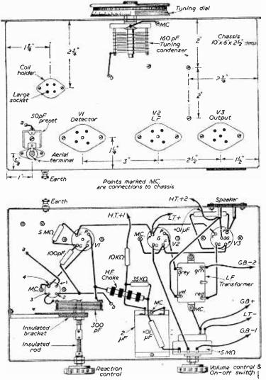
Figs. 2 and 3.—Above and below chassis wiring information. -
