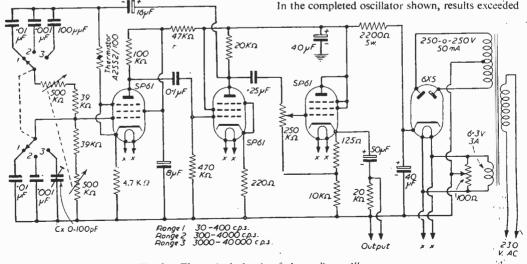
Fig. 2.—Theoretical circuit of the audio oscillator.
