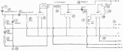
Fig. 20.—The circuit revised for applying bias to both L.F. stages.
