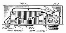
Fig. 7.-Layout and details of the aerial unit.
