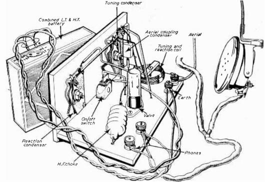
Fig. 10.—Pictorial wiring diagram of circuit shown by Fig. 1. Some of the wiring is underneath the baseboard, which is fixed to the panel to clear the valve holder sockets.
