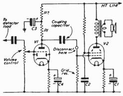
Fig. 2.—The output stage and hrst A.F. amplifier of a typical receiver.
