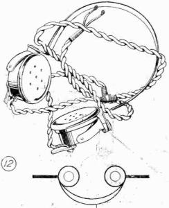
Fig. 7.-The earphone's or telephones.
