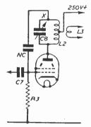
Fig. 4.—P.A. circuit using neutralisation.
