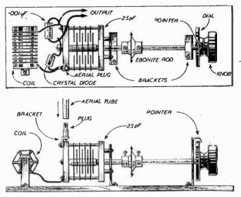
Figs. 1 and 2 .- Two views of the unit to show layout and wiring.
