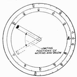
Fig. 1.—Subsidiary 'bracketing' scale for multiplier dial.
