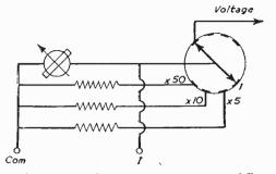
Fig. 3 .- Circuit of a current meter to give different ranges by means of a selector switch.
