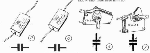
Fig. 4. (left)-Fixed, and (right)-Variable condensers.
