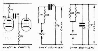
Fig. T.—Resistance-capacitance coupling circuit and equivalents for L.F. and H.F. response. (a) Actual circuit. (b) L.F. equivalent. (c) H.F. equivalent.
