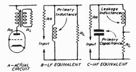
Fig. 3.—Output transformer circuit and equivalents. (a) Actual circuit. (b) L.F. equivalent. (c) H.F. equivalent.
