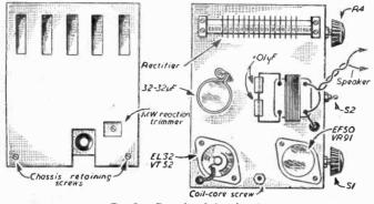
Fig. 2.—Details of the chassis.
