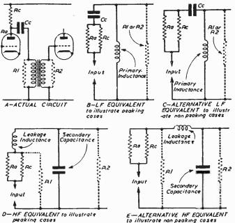
Fig. 2.—Parallel-fed interstage transformer-coupled circuit and equivalents. (a) Actual circuit. (b) L.F. equivalent to illustrate peaking cases. (c) Alternative L.F. equivalent to illustrate non-peaking cases. (d) H.F. equivalent to illustrate peaking cases. (e) Alternative H.F. equivalent to illustrate non-peaking cases.
