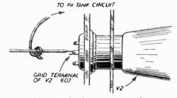
Fig. 5.—Details of neutralising condenser.
