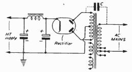
Fig. 4.—The power circuit of a normal receiver.
