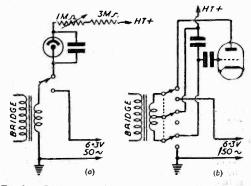
Fig. 2.-Connections for various types of oscillators.
