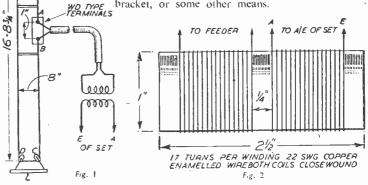
Details of the folded dipole and of the metching transformer.
