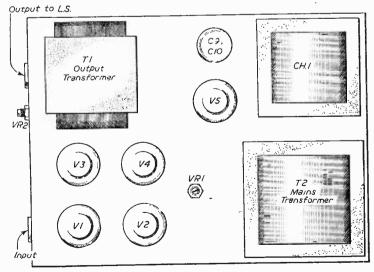
Fig. 2.—Suggested layout of the main components.
