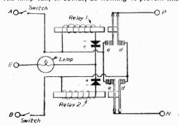
Fig. 2.—Modification for use with low-current relays.
