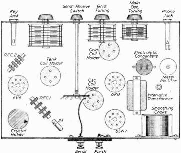
Fig. 4.—Below chassis layout.
