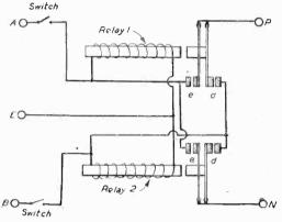
Fig. 1.—Standard circuit recommended by the author—e and depict energised and de-energised positions respectively.
