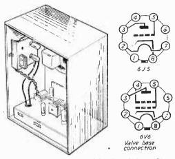
Fig. 2.—Position of amplifier in existing cabinet and valve base data.
