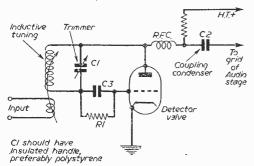
Fig. 1.—Basic self-quenched inductive circuit.
