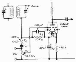
Fig. 3.—A typical pick-up input circuit of an average
