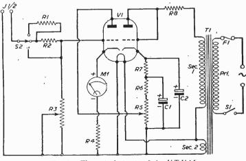
Fig. 1.—Theoretical circuit of the V.T.V.M.
