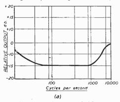
Fig. 2(a).—Approximate crystal pick-up response and (b).—Approximate magnetic pick-up response.
