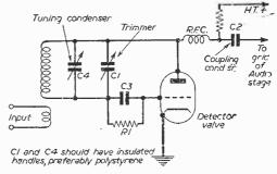
Fig. 2.—Basic self-quenched capacitive circuit
