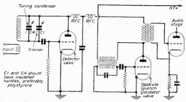
Fig. 3.—Basic externally quenched (capacitive) circuit.
