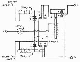
Fig. 3.—Inclusion of a third relay.
