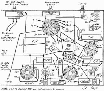
Wiring diagram below chassis of the H.F. end of the receiver.
