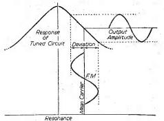
Fig. 7.—Using a mistuned resonant circuit to convert F.M. to A.M.
