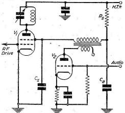
Fig. 1.—Transformer-coupled screen modulator.
