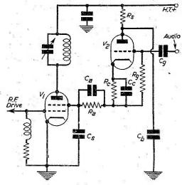
Fig. 4. \* Series-screen modulator.
