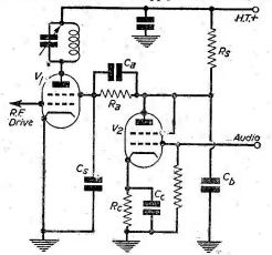
Fig. 3.—Resistance-coupled screen modulation.
