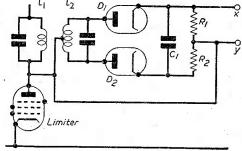
Fig. 10.—Basic circuit of phase discriminator.
