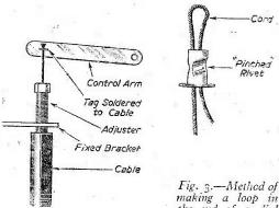
Fig. 2.—Construction of a Bowden cord adjustment.
