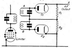
Fig. 8.—Basic circuit of amplitude discriminator.
