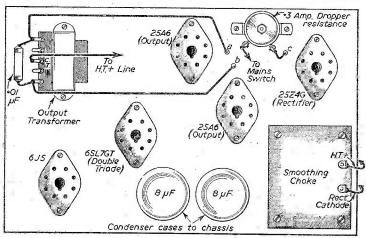
Fig. 2.—Top of chassis layout.
