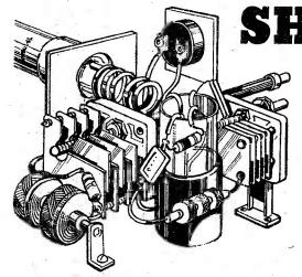
HILE we never associate wave-traps with the modern selective broadcast type superhet, this old aid to selectivity can be effectively used in conjunction with the simpler types of short-wave receiver, such as the straight detector and untuned H.F. arrangements.
