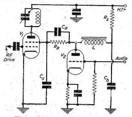
Fig. 2.—Choke-coupled screen modulator.
