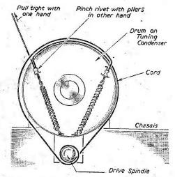
Fig. 1.—The simplest type of cord drive showing method of terminating cord.
