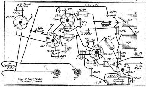
Fig. 3.—Under-chassis wiring details.
