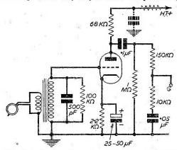
Fig. 6.—To provide bass compensation a tone-control pre-amplifier is desirable using a circuit similar to that shown here.
