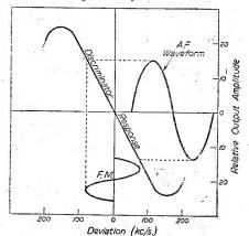
Fig. 9.—Response characteristic of amplitude discrimination.
