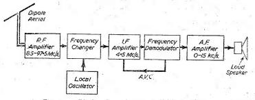
Fig. 11,—Block schematic of an F.M. receiver.
