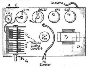
Fig. 2.-Layout of the receiver.
