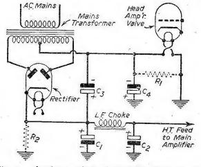
Fig. 3.—Another method of obtaining D.C. for the first value.
