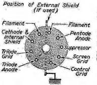
Fig. 2.—Details of value base for the ECL80 value.
