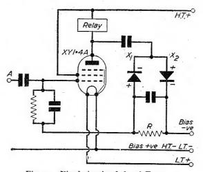
Fig. 2.—Final circuit of the A.F. stage.
