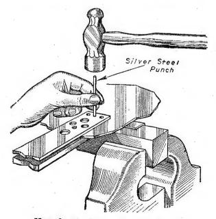
How the punch is used on the chassis.
