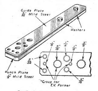
Details of construction of the punch.
