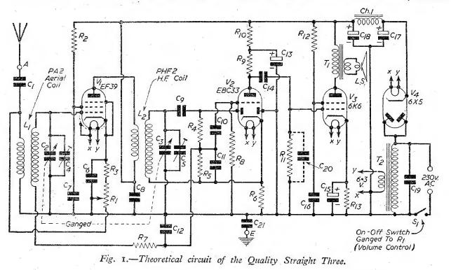
of which is connected to chassis via the On-Off switch S1. One side of the secondary of the filament transformer T2 is connected to chassis and one side also of all filaments. C19 acts as a filter across the mains and should be a good quality component. Note that as one side of the mains is connected to chassis the set must always be earthed via a condenser (C21).
