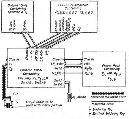
Fig. 4.—Unit block diagram of the amplifier. The parts are shown in Fig. 3.
