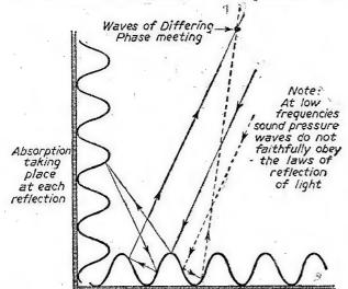
Fig. 2.-Part cross-section of lined cabinet showing possible paths of sound waves from loudspeaker.
