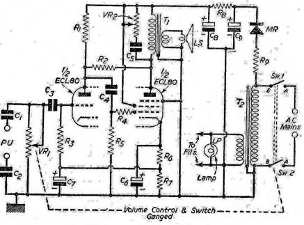
Fig. 1.—Theoretical circuit of the amplifier.
