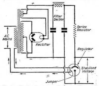
Fig. 3.—Circuit of a mains unit showing "jumper" connection.
