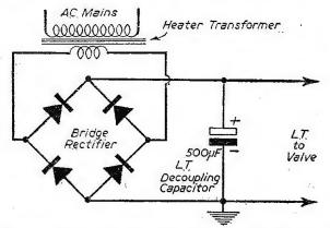
Fig. 1.—Method of obtaining D.C. for the first valve, using a Bridge Rectifier.
