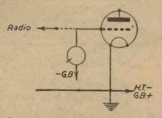
Fig. 1.—Normal connections for a pick-up with a battery-operated triode.
