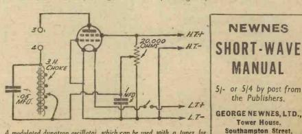
A modulated dynatron oscillator, which can be used with a tuner for wavelength checking, or for adjusting the trimmers in a set having ganged tuning condensers.
