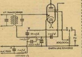
Fig. 3.—The single-diode-tetrode for A.V.C. and gramophone reproduction. The arrangement shown is suitable for use in a superhet. Connections to anode and screen are normal. An H.F. filter may be necessary at "x" in certain circuits. Components marked \* are liable to modification. Value of bias resistor varies widely with different makes of value. That recommended by value maker should be used. 155
