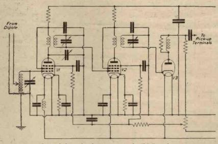
A typical three-value short-wave circuit for T.R.F. working.
