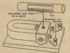
An improvised counter for fine coil windings.
