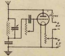
Fig. 9.- The Ultra-Audion, a tricky but interesting single-valve " super " circuit.
