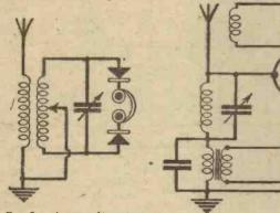
Fig. 2.- A crystal' receiver using full-wave rectification.
