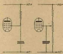
Fig. 1.—Alternative methods of feeding the screen-grid of a pentode value.
