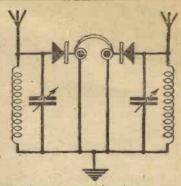
Fig. 1.- A simple circuit for obtaining increased volume from a crystal set.
