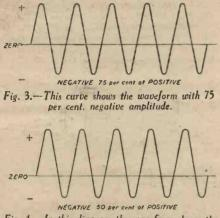
Fig. 4.—In this diagram the waveform shows the negative half-cycle 50 per cent. of the positive.
