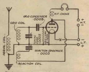
The basic circuit of a one-valver which can be used for experimental purposes.
