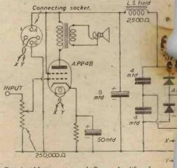
Fig. 4.-Mains section and Power Amplifier for use Receiver.
