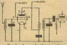
Note how the second grid is inserted in the S.G. valve.
