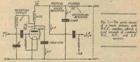
condenser as shown, but an alternative method is to use a differential condenser for reaction control, as shown in Fig. 2. In that case, the capacity to earth remains constant regardless of the setting of the reaction condenser. There is, of necessity, some slight variation in effective H.F resistance between the anode and earth, because of the reactance of the reaction winding, but this is of little practical importance.
