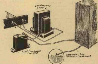
Method of connecting a loudspeaker when it is to be used at a distance from the set.
