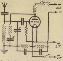
Fig. 6.—Circuit of the Armstrong Superregenerative single-valver.
