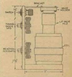
Fig. 3.-Side view, showing value-holder bracket which supports the L.F. valve within the coil.
