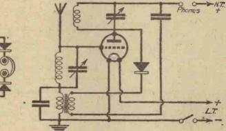
Fig. 4.-- An early form of valve-crystal reflex circuit.
