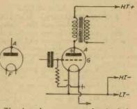
The electrode arrangements for the diode (left) and the triode (right) are shown here.
