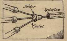
An effective method of making multiple connections
