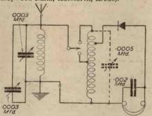
Circuit diagram of Mr. A. S. Long's crystal set. Wave Trap Coil; 60 turns 30 S.W.G. enamelled copper wire on a former 1½, in. diameter. Aerial Detector Coil; 76 turns of 30 S.W.G. enamelled copper wire on a former 21 in. diameter. Crystal tap at 10 turns. Aerial tap at 40 turns. Variable condensers preferably ganged, 0003 or .0005 mfd. The .0005 tuning condenser is not required, as in the 150 mile circuit, the wave-trap serves the same purpose.
