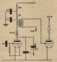
Fig. 4.—Double-decoupling added to the anode circuit of the original detector stage.
