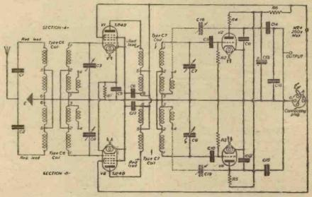
Fig. 1.-Theoretical circuit diagram of the diversity receiver described on this page.
