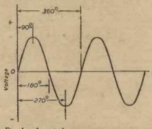
Fig. 1.—A typical sine curve representing an alternating voltage.
