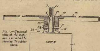
These parasitic vibrations can be prevented largely from reaching the turntable by interposing a vibration absorbing member between the turntable and its driving spindle. A soft-rubber sleeve may, for example, be fitted over the turntable spindle, and the turntable mounted on this sleeve. A suitable form of sleeve is shown in plan, in elevation and in vertical crosssection in Figs. 2, 3 and 4, and a gramophone motor unit complete with sleeve is shown in Fig. 1.
