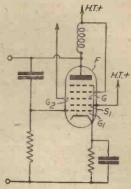
Fig. 2.- A five-grid value for the special arrangement described here.
