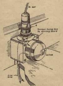
A safety mains-plug switch attached to a skirting board.
