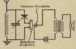
Fig. 3.—The arrangement of a microphone amplifier for operating a loudspeaker from a crystal set.
