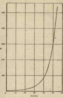
Fig. 1.-Graph showing the gain or loss ratios in relation to decibel equivalents.
