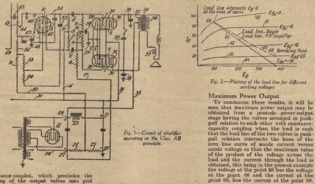
resistance-coupled, which precludes the driving of the output valves into grid eurrent. The anode resistors for the phase inverter may be 100,000 ohms with coupling capacitors of 0.01 mfd. and grid resistors of 270,000 ohms. The bias for the push-pull output stage is obtained from the two resistors in series in the H.T. negative lead.
