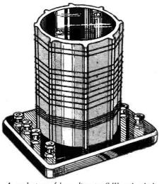
An early type of large-diameter S.W. coil, which is a good example of spaced windings.
