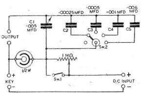
Fig. 1.-Wiring diagram of the simple Neon-tube test unit. Either batteries or external power pack may be applied.
