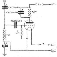
Fig. 1.—Two condenser positions for series tuning, and a tuned reaction circuit.
