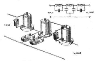
Fig. 9.—One arrangement of gramo-scratch filter.
