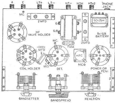
Fig. 3.-Diagram showing layout of chassis components.
