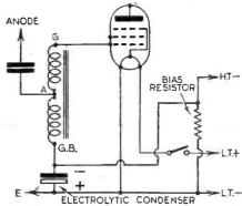
Fig. 2.—Automatic grid-bias is always to be preferred. Connections shown here refer to a parallel-fed transformer arrangement, supplying a pentode.
