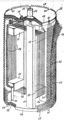
Fig 2.—Constructional details of the frame aeria!.
