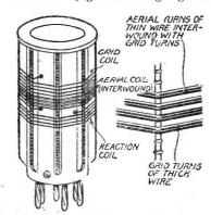
A modern type of S.W. coil showing aerial, grid and reaction windings.
