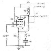
Fig. 4.-A circuit arrangement incorporating the modifications described.
