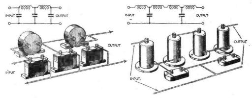
Fig. 8.-Alternative arrangement of multiple filters.
