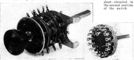
Figs. 9 and 10.—The rotary wave-change switch in two different patterns Connections and methods of operation of the model on the left are shown in Fig. 11 and for the switch on the right in Fig. 12.
