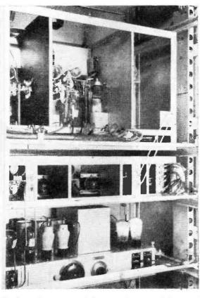
The form taken by a crystal drive unit of a modern high-powered television transmitter working on ultra-short waves.
