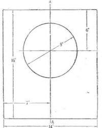
Fig. 6.—Details of the recommended speaker cabinet design.
