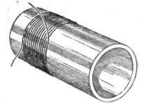
Fig. 2.—An example of single layer solenoid winding not difficult to construct.
