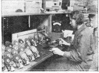
Statistics reveal that three out of every five radio employees are testers. The above illustration shows a tester checking motor-driven wavechange switches in the Ekco factory.
