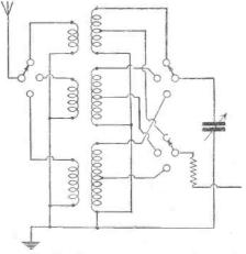
Fig. 2.—How to arrange wave-change switching
