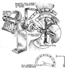
A simple mechanical bandspread drive.
