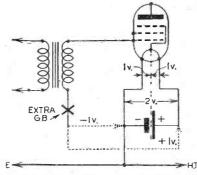
Fig. 1.—It is possible to use the voltage drop across the filament to provide a small amount of bias—although not half the L.T. voltage.
