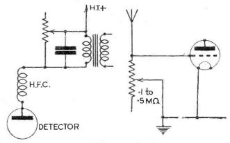
Figs. 3 (left) and 4 (right).—Volume control at detector output, and aerial volume control.
