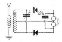
Fig. 4.—One of many full-wave-detector circuits which were tried with little success.
