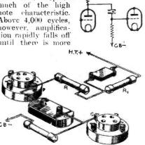
Fig. 3.-A bass booster for an R.C. coupled circuit.
