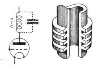
Figs. 1 and 3.—Self-capacity can be likened to a small condenser across the winding, as shown on the left. A typical slotted former often used for the winding of the L.W. section is shown on the right.
