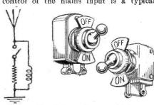
Fig. 5 .- A" local-distance" switch and the circuit arrangement.
