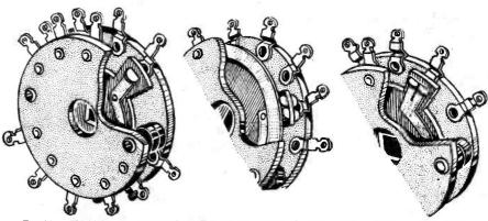
Fig. 11.—How the rotary switches (Fig. 9) are designed. Three different patterns are shown.
