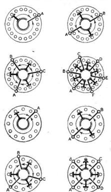
Fig. 12.—Connections available for the type of switch shown in Fig. 10.
