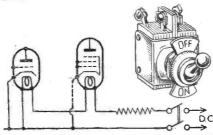
Fig. 7.-In a D.C. receiver both mains leads should be operated, and a Q.M.B. double-pole switch of the type indicated should be used,
