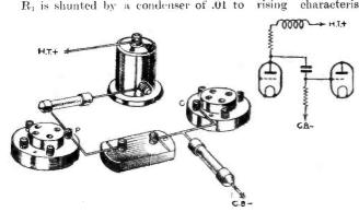
Fig. 4.—The arrangement for a simple treble booster.
