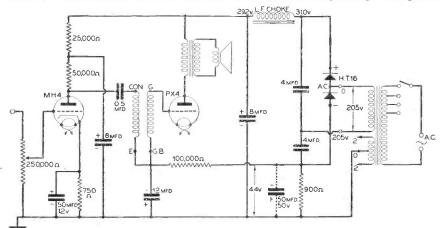
Fig. 1.—Theoretical circuit diagram of the amplifier.
