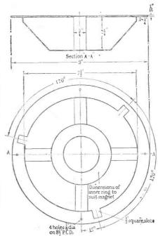
Fig. 7.—Suggested construction of the speaker frame,
