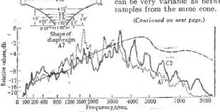
Fig. 5.-Comparison of diaphragms C2 and A7.
