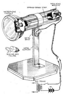
An old torch case is utilised for making this microphone.
