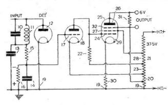
Fig. 1.-A circuit incorporating a tuned input and a limiter arrangement as described in the text.
