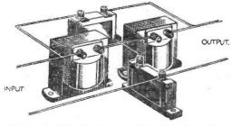
Fig. 7.—A low-pass filter for eliminating heterodyne whistles in the output stage.
