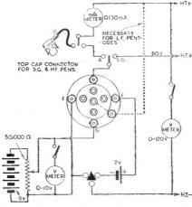
Fig. 1.—A suggested circuit for a simple valve tester. Refinements can be added to suit requirements.
