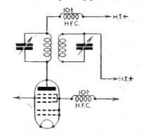
Small, 10-turn H.F. stopper chokes will often prevent instability when wired in the anode and/or screening grid circuit of a frequency changer or H.F. pentode.
