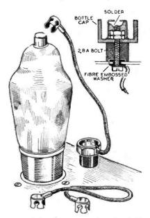
A method of ensuring safety for T.C. connections.
