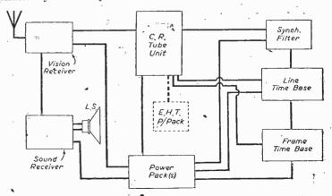
Diagram showing the general arrangement of a modern television picture and sound receiver.
