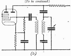
Fig. 4.—On the left (a) is a direct grid-timed oscillator circuit, and on the right (b) the anode circuit is tuned.
