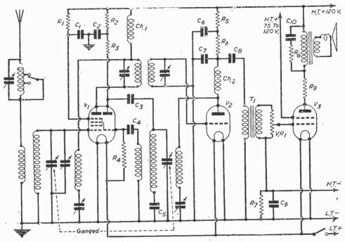
Fig. 2.—Battery version of a circuit on the lines of Fig. 1.
