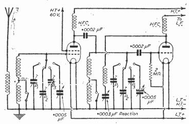
Fig. 2.—The same type of switch is used in this circuit, but manual tuning is provided and a reaction circuit is included.
