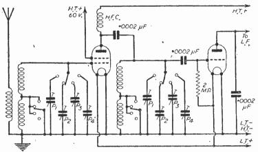
Fig. 1.—A simple two-valver with a rotary 4-position switch assembly to provide choice of four stations.
