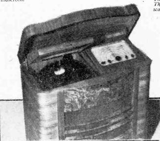
The Ether Conqueror, type K.129R, made by Dynatron, is fitted into a Regency cabinet, and as may be seen has a special lid for the record reproducing section, and a sloping panel on the radio side.
