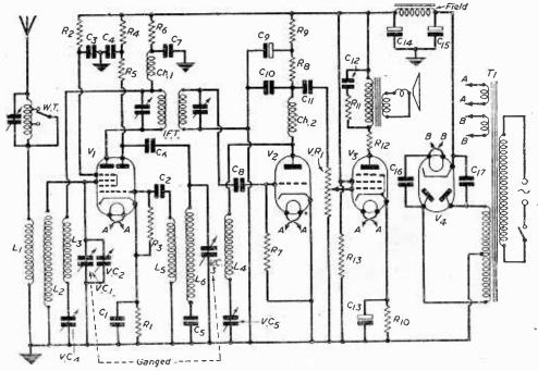
Fig. 1.—A.C. Mains Short-wave Three as described.
