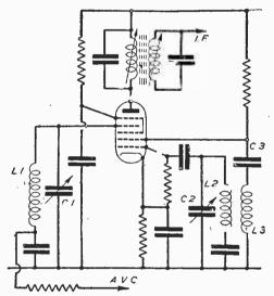
Fig. 1.—A typical modern frequency-changing stage.
