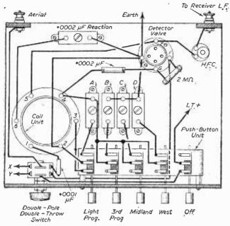
Fig. 7.—Practical layout for a push-button operated single valver.
