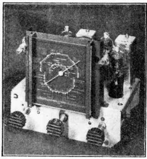
The R.M. "Radio Feeder," a three-waveband three-valve unit for addition to a standard power supply and amplifier.
