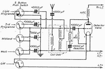
Fig. 3.—Push-button switching in its simplest form is indicated in this circuit diagram.
