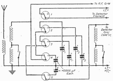
Fig. 5.—Utilising one of the push-buttons for on-off switching purposes.
