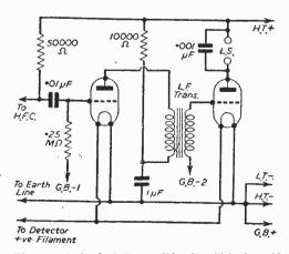
Fig. 4.—A simple L.F. amplifier in which the grid resistance of the first stage may be replaced by a variable component to provide volume control.
