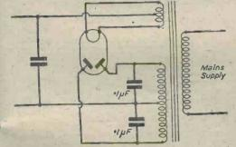
Fig. 7 .- Cure for modulation hum when the rectifier circuit is to blame.
