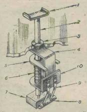
Details of a pickup rest with an on off switch incorporated.
