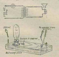
Circuit diagram and complete unit for centring speaker cones.
