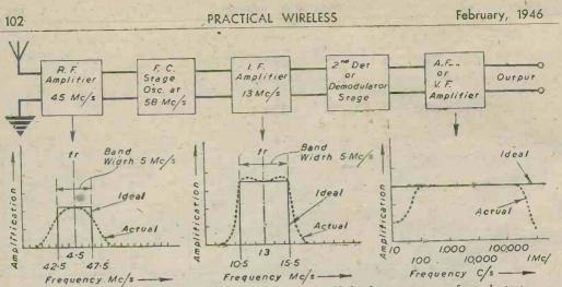
Fig. 2 .- Block diagram of ultra-short wave receiver with wide-band response curves for each stage.
