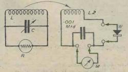
Fig. 2.-Artificial aerial circuit diagram.
