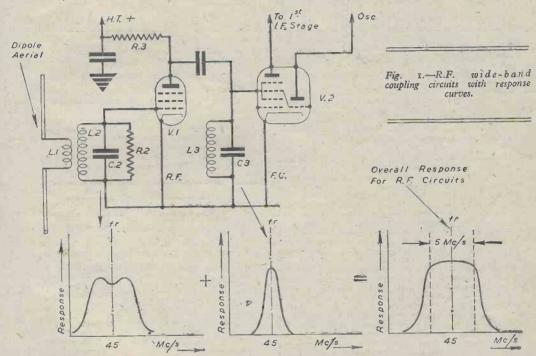
cuits of the familiar broadcast receiver are modified and developed to meet the requirements of television and frequency modulation reception.
