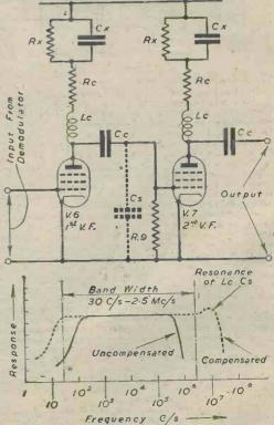
Fig. 3 .- Two-stage video amplifier with response curve.
