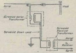
Fig. 4.-Connections of commercial " anti-static " aerial.
