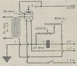
Fig. 6.-Addition to auto-bias circuit.
