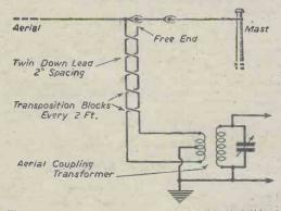
Fig. 5.—Transposed feeder for short-wave reception.
