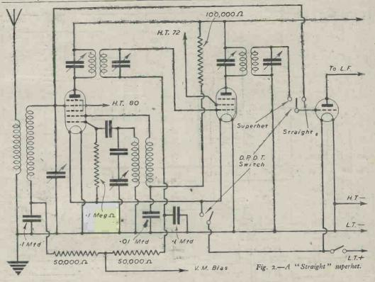
is connected and also the coupling condenser is connected to the valve grid. Results are then normal. In the other position the valve filament is disconnected and the connection from the coupling condenser transferred
