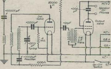
Fig. 1.—Theoretical circuit.
