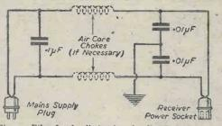
Fig. 3.—Filter for the elimination of radiated interference.
