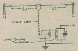
Fig. 6 .- An anti-noise aerial which works well on shortwaves.
