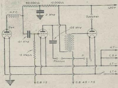
Fig. 3.-Circuit with switching for L.S. and 'phones.
