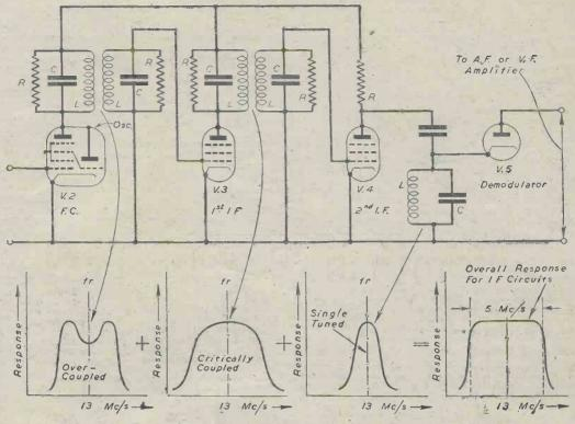
Fig. 4.-I.F. wide-band coupling circuits with response curves.
