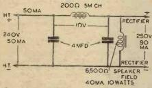
Fig. 5.—A 6,500-olim speaker-field connected in parallel with the H.T. supply in an A.C. or D.C. receiver.
