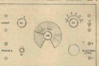
Fig. 2.—Panel layout of the complete meter.
