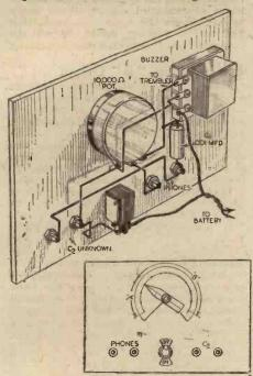
A simple but efficient capacity bridge.
