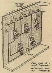
use individually or collectively. By operating the switches when two or more speakers are joined rapid comparisons are possible for test purposes, or if the speakers are fed from a distant point individual rooms may be switched in and out as required.
