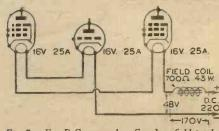
Fig. 7 .- For D.C. sets only. Speaker field in the heater circuit. Few speakers could take the 38 watts indicated without overheating, but the circuit could be modified to overcome this difficulty by using a field of lower resistance in series with a resistor.
