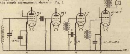
Fig. 2.—Skeleton circuit diagram showing various ways of biasing indirectly-heated valves.
