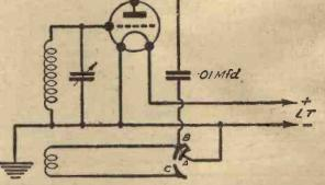
Fig. 3.—Simple connections for an automatic tone balance circuit.
