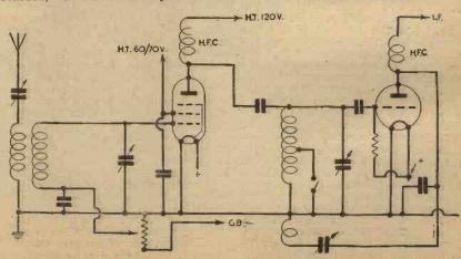
Fig. 2.—The theoretical circuit of a tuned grid H.F soupling which is the method used in this unit.
