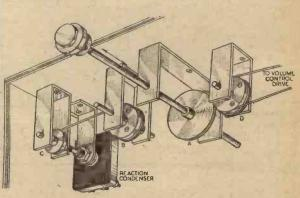
A simple dodge for driving two components from a single spindle.
