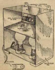
A novel device for the heat treatment of damp
