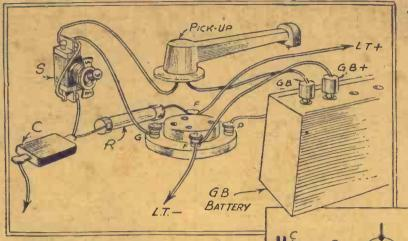
Connecting a pick-up permanently to a battery detector stage.
