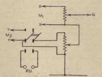
Fig. 2.—Shows how to introduce a P.U. when required by switching.
