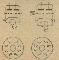
Fig 2.—Theoretical diagrams of the 6N7G and 6C8G valves and under-valveholder view of pin connections.
