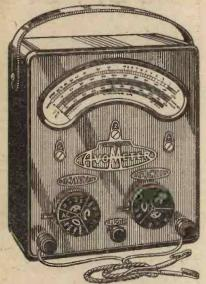
The Avo Test Meter. which has several separate ranges, easily selected by rotary switches.
