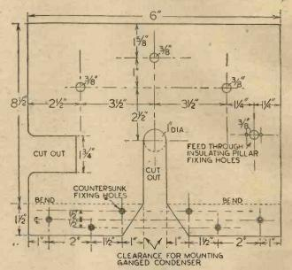
Figs. 4 (left) and 5 (above).—Details of the chassis and vertical mounting screen.
