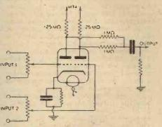
Fig. 5.—Using a double-triode as an input mixer for two "mikes" or pick-up.
