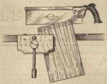
Fig. 3.—When making a corner halving the cut down the grain should be made first.
