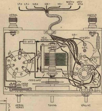
From the above diagram the layout and all wiring can be obtained, while on the left the panel dimensions, are shown.
