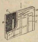
As applied to a tuning scale for a wireless receiver, a front transparent plate A of glass, mica synthetic or material (see accompanying illustration) has the scale indicia, D, E, printed on its
