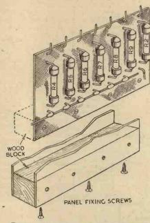
Fig. 4.—How the resistance strip is mounted.
