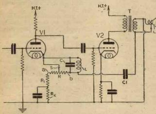
Fig. 1.-A two-stage amplifier with negative feedback.
