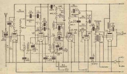
Fig. 1.—Theoretical circuit diagram of the Short-Wave Five.
