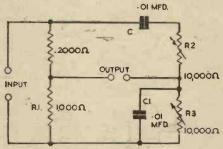
Fig. 2.—Circuit values for the heterodyne filter.
