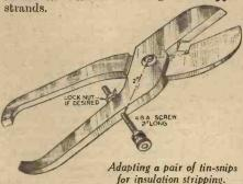
On each blade, about one inch from the rivet, file a notch, using a three-cornered file. These two notches should be of such a depth so that, when the cutters are closed, the apex of each notch just covers the other. Both must be carefully bevelled to leave sharp cutting edges. In the side of one handle, about two inches from the rivet, drill a hole and tap 4BA. A two-inch length of 4BA screwed rod, which can have a terminal head locked on one end, is screwed into the hole.
