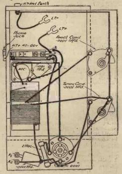
long-at the end being fixed a small accumulator spade, which is for connecting to the plus side of the accumulator. There now remains a black banana socket; this is mounted towards the back of the righthand side of the box. To a 4in length of rubber-covered wire is fastened a black accumulator spade, and it is soldered to (Continued on page 250)
