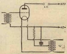
Fig. 3.—Diagram showing the bias scheme for a directly-heated valve.
