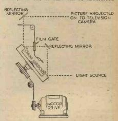
Fig. 2.—The light and picture paths shown simply for the film projector used in television transmission.
