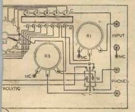
Fig. 3.-Wiring diagram of the meter.
