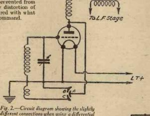
different connections when using a differential reaction condenser.
