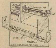
Insulated coupling brackets for extension rods.
