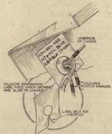
A method of marking battery leads.
