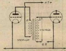
A class B transformer steps down, because the valve is power operated; an ordinary L.F. transformer steps up because the L.F. valve is voltage operated.
