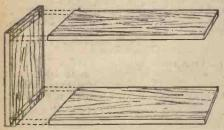
bottom. After that, a front panel can be fixed with nails or screws, and a back made which can easily be removed. As an alternative, it might in some instances be preferable to fix the back, leaving the front open so that a chassis, with its own metal or plywood front panel, can be slid into position. It is desirable, in any event, to make either the back or front a fixture, because this will stiffen the assembly to a marked degree.
