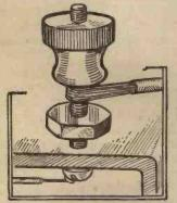
Flex must be carefully handled when used beneath terminals, as loose strands can give rise to noisy backgrounds.
