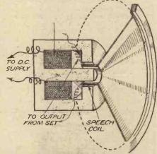
Fig. 2.—Sectional diagram showing the construction of an energised speaker. Compare with Fig. 1.
