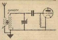
The step-up effect of an H.F. transformer is limited, due to the capacity between primary and secondary windings, and the number of turns required on the primary,
