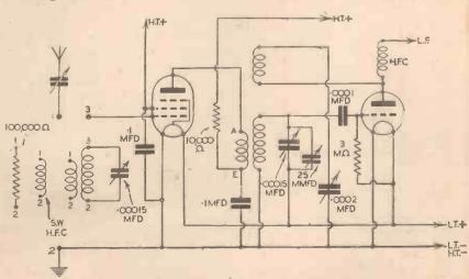
Fig. 2.—Connections for an H.F. amplifier with alternative aerial-circuit connections. Aperiodic tuning is provided by the resistor or H.F. choke, whilst a four-pin coil and variable condenser give better selectivity.
