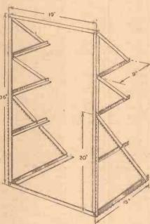
Fig. 2.—The general details for the construction of a serviceable metal rack.
