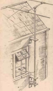
A method of mounting a rotatable horizontal beam aerial of simple design.
