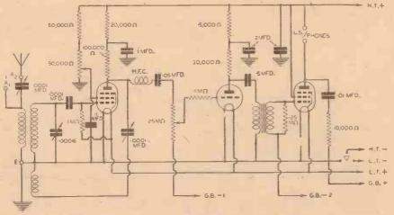
Fig. 1.—Theoretical circuit diagram for the first part of the Kestrel S.W. Four.
