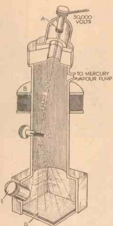
Sectional view of an electron diffraction camera, showing the interior construction.
