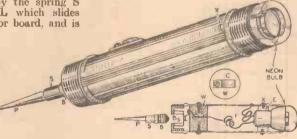
A handy neon test prod, and section showing construction.
