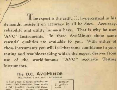
A high-grade 13-range combination meter, this instrument incorporates a fully jewelled moving-coil movement which ensures accurate readings. Its 13 ranges are adequate for the majority of circuit, battery and resistance tests. The total resistance of the meter is 100,000 ohms; full scale deflection of 300v. or 600v, is obtained for a current consumption of only 3 mA. and 6 mA. respectively.
