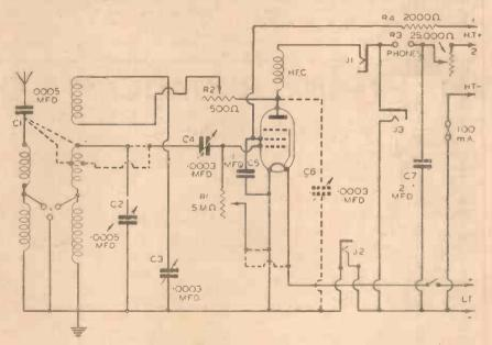
Fig. 1—The circuit employed. Note the use of several variable components and the inclusion of jacks for current and voltage readings.
