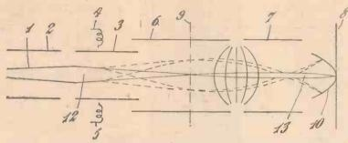
Fig. 1.—The path of the electrons is depicted above, the screen being represented by &.
