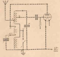
Fig. 7.—The connections for the Lucerne Coil are shown here and it will be seen that it can be used for many circuits.
