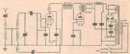
Fig. 11.—The theoretical circuit of the Economy A.C. Two. A modern coil can be used as mentioned in the article.
