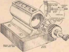
A coil-winding counter made with an old cyclometer
