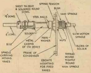
An adapted slow-motion driving head and extension rod.
