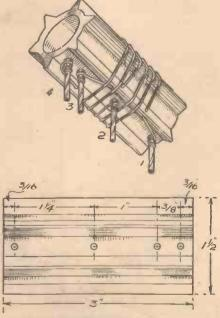
Fig. 9.—The winding of the S.W. coil is not difficult if these diagrams are studied. Drilling holes are clearly indicated.
