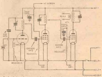
Fig. 2.—A three-valve transmitter of the simplest type. It is open to many modifications and is ideal for the A.A. licence holder.
