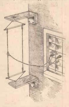
A simple vertical aerial, with reflector, may be arranged on the lines shown here.
