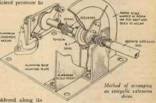
length of quarter-inch brass rod fitted into the end of the epicyclic drive. Aluminium of 16 S.W.G. is used throughout for the mounting, but to prevent the capacity of the condenser being exceeded, this mounting bracket, as depicted by the dotted lines, does not cover the plate of the condenser. The
