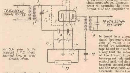
its value at cut-off to its value at any given set of operating voltages; T2 is the transit time from control-grid to screen-grid; time from control-grid to screen-grid; T<sub>1</sub> is the transit time from cathode to control-grid; k is the square root of the ratio of the effective voltage at the screen-grid-to that at the control-grid; and C<sub>c</sub> is the capacity between such sections of con-trol-grid and cathode as are in the electron stream.
