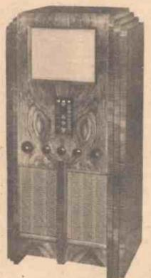
Baird's new television receiver, Model T.25, giving a picture size of 10in. by 8in.
