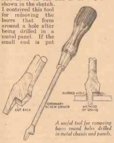
down in the hole and pressed tightly, and the handle turned round two or three times, it will take the burrs off flush with metal.—D. Robinson Co. Down).
