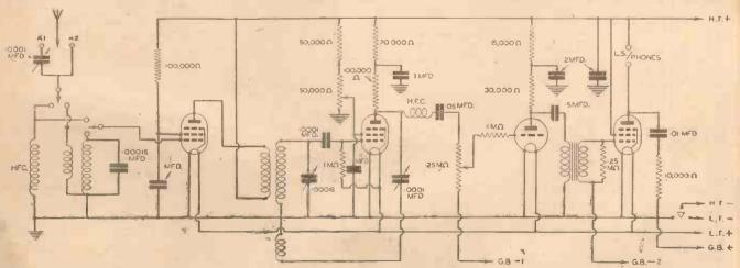
Fig. 1.—The theoretical circuit of the complete four value receiver. It should be noted that the condenser across the aerial coil is, of course, a variable, and not a fixed as shown.
