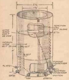
Fig. 6.—The main constructional details of the Lucerne Coil are shown above.
