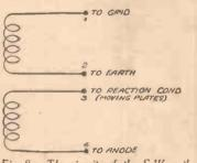
Fig. 8.—The circuits of the S.W. coil shown in Fig. 9.
