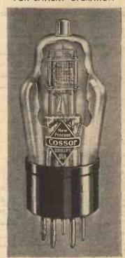
The new Cossor 220 I.P.T. is a special Pentode Detector Valve designed for use in Battery Receivers. Due to its indirectly heated cathode it has remarkable antimicrophonic properties even under very adverse conditions. It is, therefore, particularly suitable for use in Portable Receivers where high L.F. gain is usually provided. The base used on the 220 I.P.T. is of the 7-pin type with standard H.F. Pentode connections.
