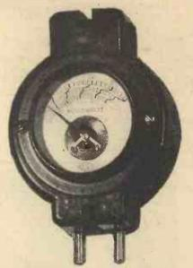
A useful wattmeter manufactured by Messrs. Bulgin.
